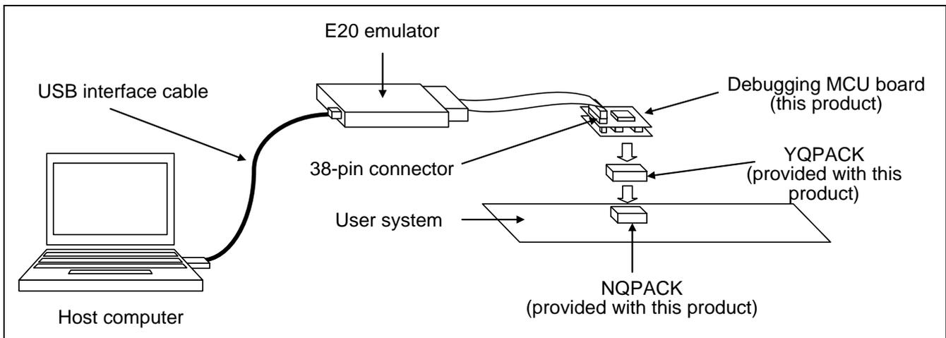
Figure 1 System Configuration
