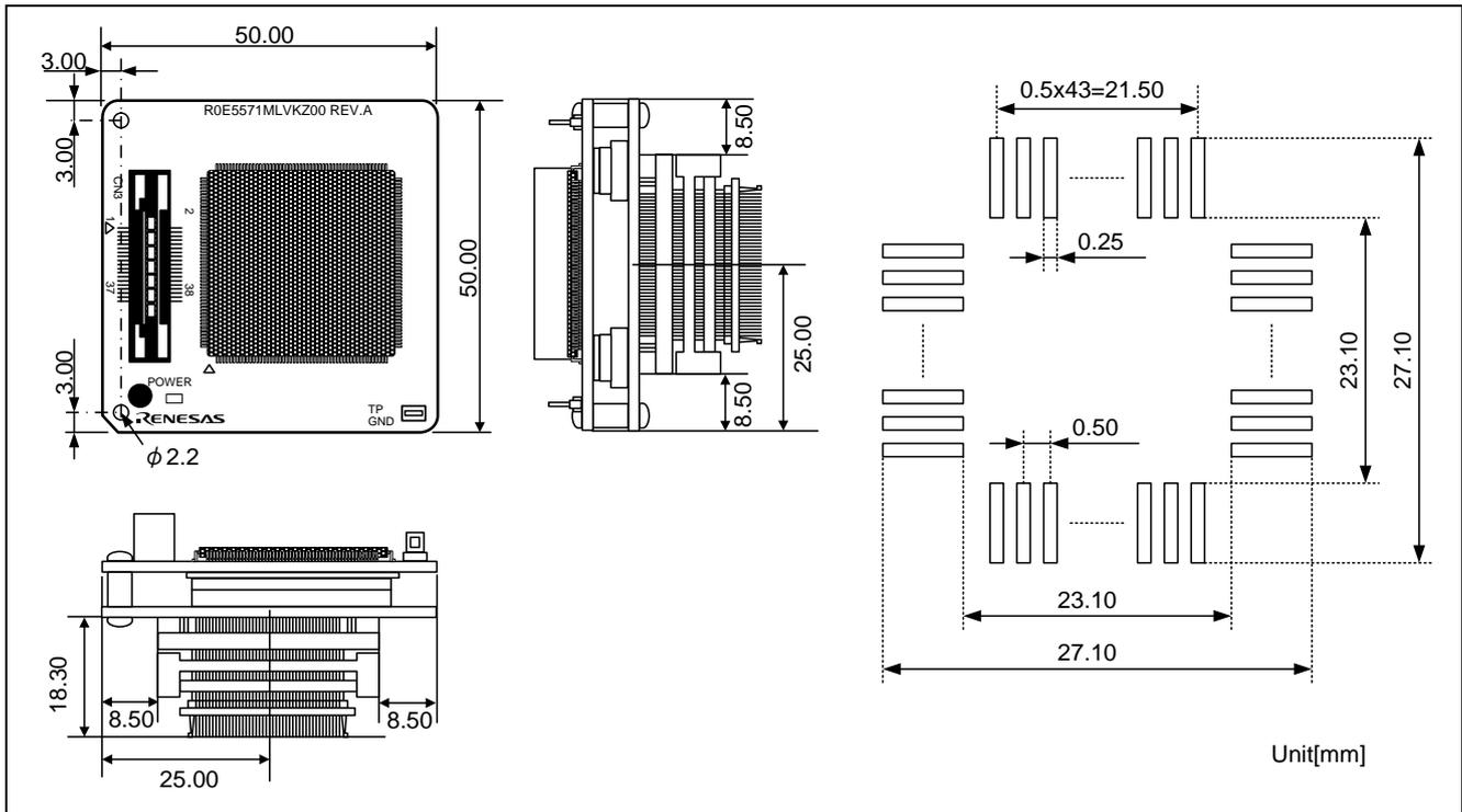
Figure 4 Reference Foot Pattern and Dimensions of This Product (R0E5571MLDMB00)
