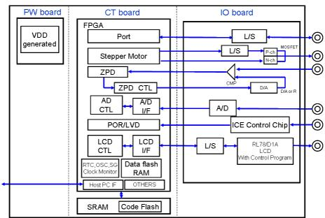
Figure A-1. Overview of QB-RL78D1A Block diagram
