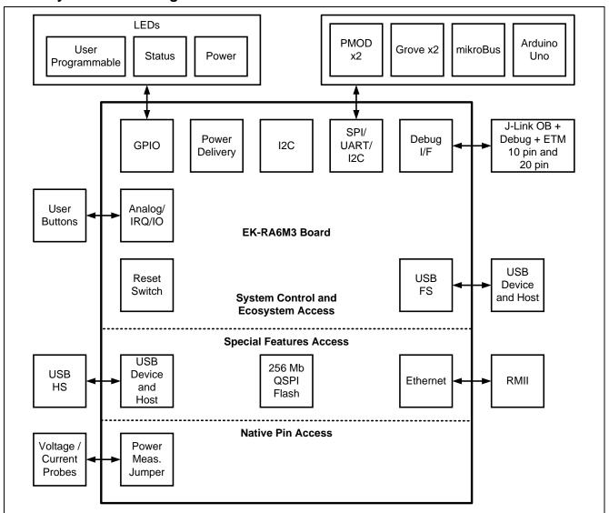
Figure 5. EK-RA6M3 Board Block Diagram
