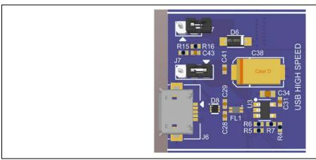
Figure 22. USB High Speed Connector
