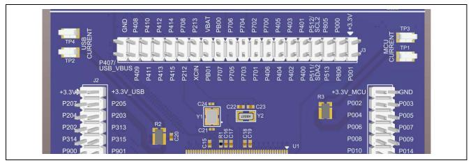
Figure 27. RA MCU Current Measurement
