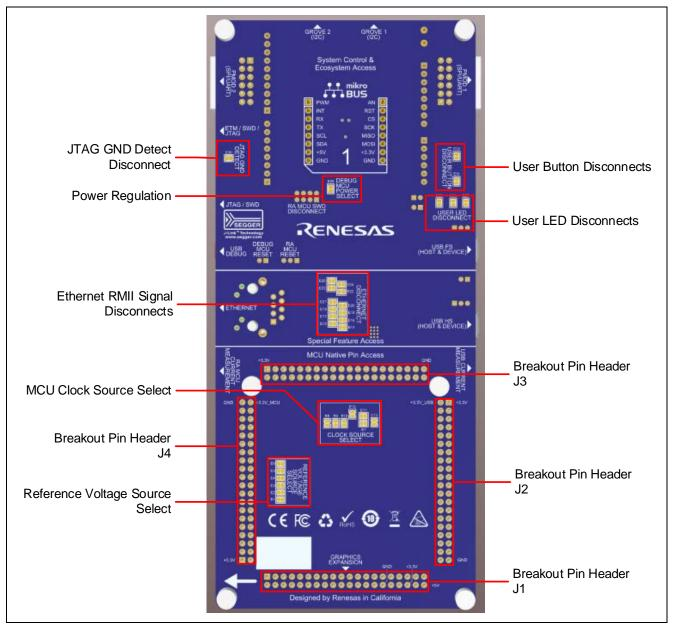
Figure 2. EK-RA6M3 Board Bottom Side
