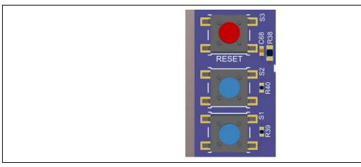
Figure 18. Reset and User Switches
