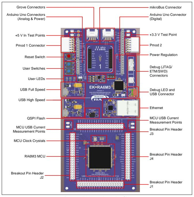
Figure 1. EK-RA6M3 Board Top Side
