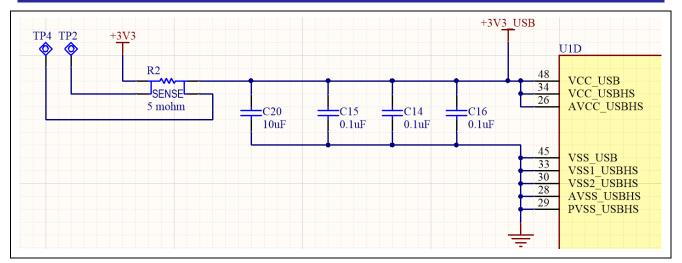
Figure 25. RA USB Current Measurement Circuit
