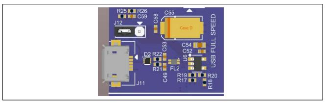
Figure 15. USB Full Speed Connector
