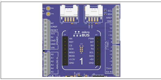
Figure 13. Arduino Uno Connectors
