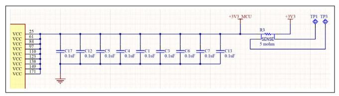
Figure 26. RA +3.3 V Current Measurement Circuit
