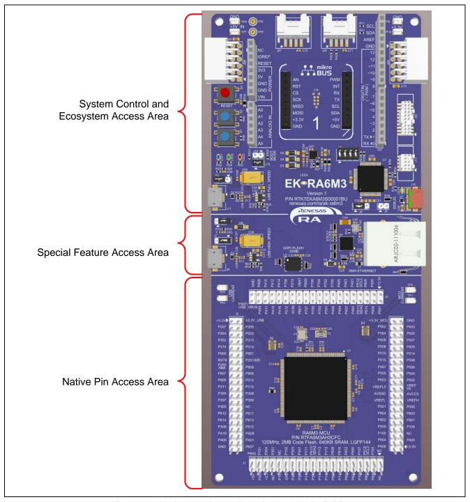
Figure 4. EK-RA6M3 Board Functional Area Definitions
