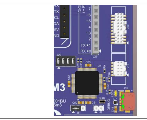
Figure 9. EK-RA6M3 Debug Interface
