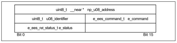
Figure 5-2 Alignment of Variables of the Request Structure (st\_ees\_request\_t)
