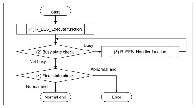
Figure 5-5 Command Operation Flowchart
