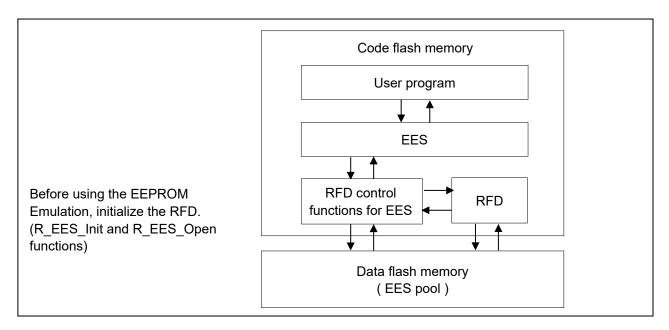
Figure 2-1 System Configuration
