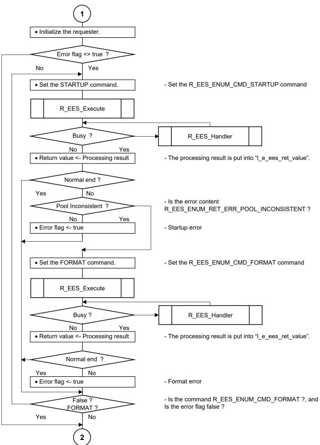
Figure 6-4 Flowchart of Sample Processing for Controlling EEPROM Emulation (2/5)
