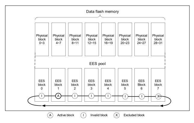
Figure 3-1 EES Pool States Example (The EES block size is set to 1 Kbyte)
