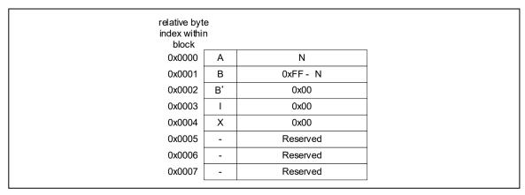
Figure 3-4 Structure of EES Block Header
