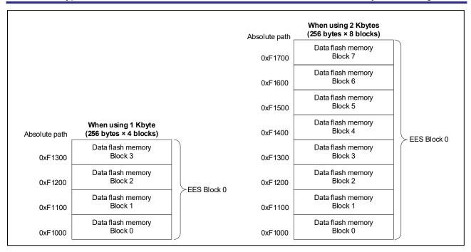
Figure 2-2 Schematic diagram of EES block 0
