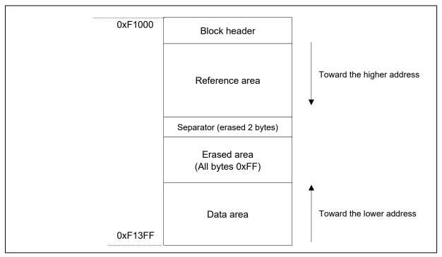
Figure 3-3 EES Block Structure(1 Kbyte)
