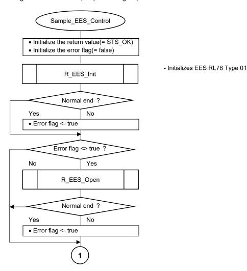
Figure 6-3 Flowchart of Sample Processing for Controlling EEPROM Emulation (1/5)
