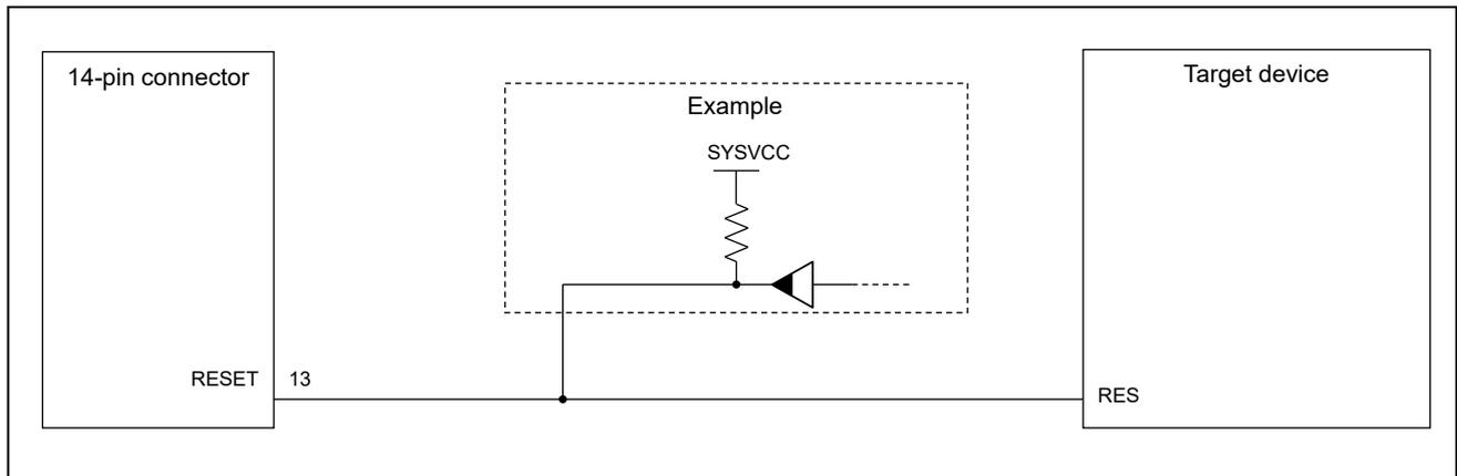
**Figure 2-6 Example of Connecting a Reset Circuit**
