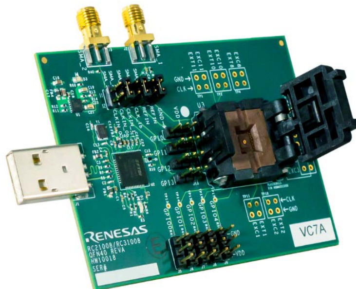
Figure 1. RC21008A/RC31008A Programmer Board
