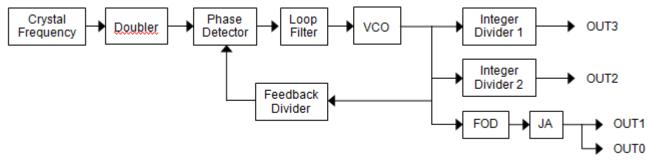
"FOD" is Fractional Output Divider and "JA" is Jitter Attenuator for use with Spread Spectrum only.
