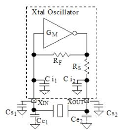
Ci1 and Ci2 are on-chip capacitors that are programmable.
