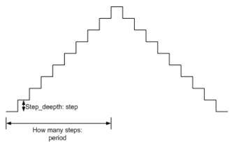
The SS modulation Period is defined as the amount of time steps it takes for the triangle to move from its lowest to its highest point. The Period is essentially half of the modulation cycle or modulation rate. One time step is defined as one cycle of the output frequency FOUT. The Period register setting needs to be half of the Period decimal value so essentially ¼ of the modulation cycle.
