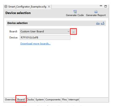
Figure 4-1 Selecting the Device
