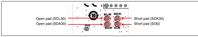
Figure 5-2 Positions of Open and Short Pads (Pmod<sup>™</sup> 1) (Soldered Side)
