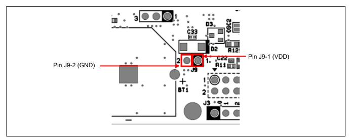
Figure 5-19 Positions of the External Power-Supply Header (Top Side)
