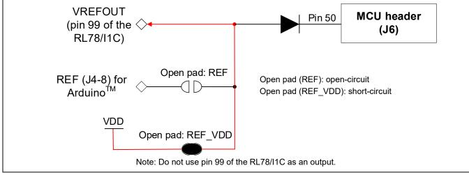
Figure 5-27 Circuit Schematic when VDD is Selected
