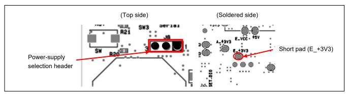
Figure 5-16 Settings to Select the Use of +3.3 V (Short Pad (E\_+3V3))
