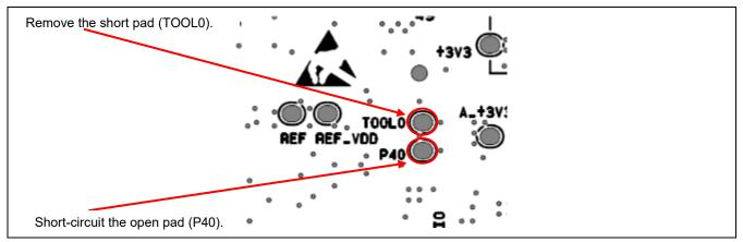
Figure 5-11 Positions to be Modified when P40 is to be Connected to the MCU Headers (Soldered Side) (\*2)
