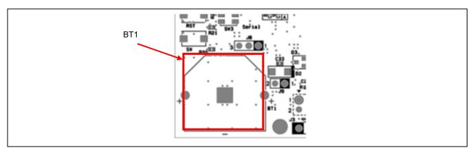
Figure 5-20 Position of BT1 (Top Side)
