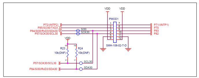
Figure 5-3 Circuit Schematic of Pmod™ 1
