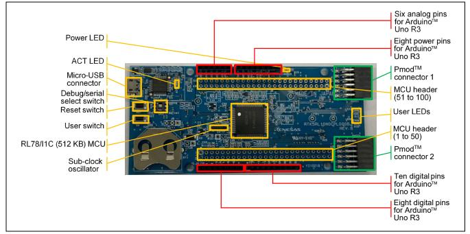
Figure 2-1 shows the external appearance of the top side of this product.
