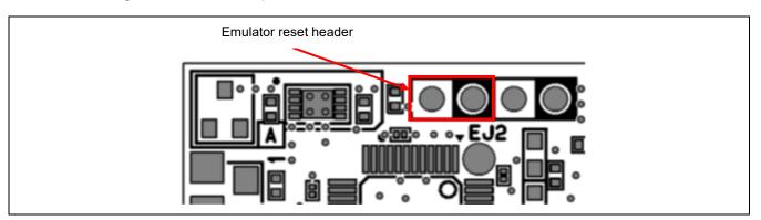
Figure 5-15 Position of the Emulator Reset Header (Top Side)
