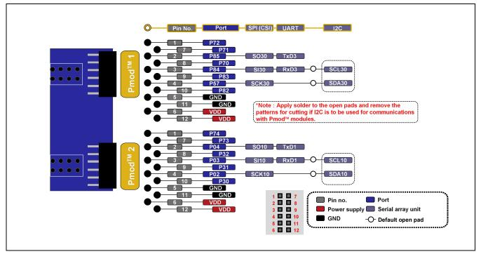
Figure 5-1 Pin Assignments of the Pmod™ Connectors
