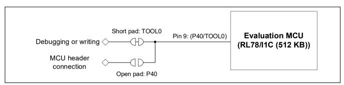
Figure 5-10 Block Diagram of Switching between TOOL0 and P40 (\*2)
