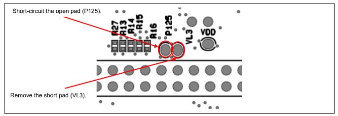
Figure 5-13 Positions to be Modified when P125 is to be Connected to the MCU Headers (Soldered Side) (\*3)
