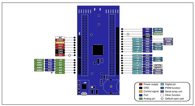
Figure 5-6 Pin Assignments of the Arduino™ Connectors
