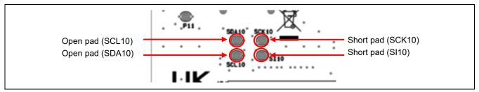
Figure 5-4 Positions of Open and Short Pads (Pmod<sup>™</sup> 2) (Soldered Side)
