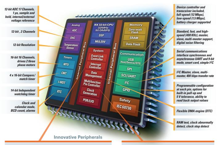
The **Event Link Controller (ELC)** is an innovative way to reduce CPU load by directly routing interrupt event signals from one peripheral or module to the other; as a result, power consumption, interrupt latency and program size are minimized.
