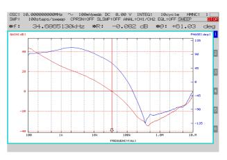
Figure 16. 24V<sub>IN</sub>, 2A, Fc = 35kHz, PM = 61° at 85°C
