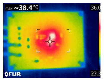
Figure 21. Thermal Image 24V<sub>IN</sub>, 3.3V<sub>OUT</sub>, 400kHz, 2A HTSSOP Package, IC Temperature at 38.4°C
