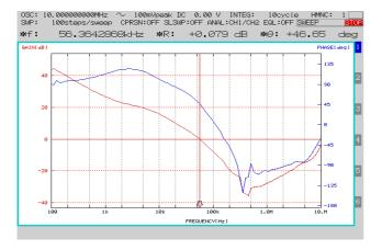
Figure 17. 24V<sub>IN</sub>, 2A, Fc = 56kHz, PM = 47° at -40°C
