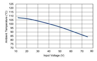
Figure 19. Derating Curve: 3.3V<sub>OUT</sub>, 400kHz, 2A, QFN Package
