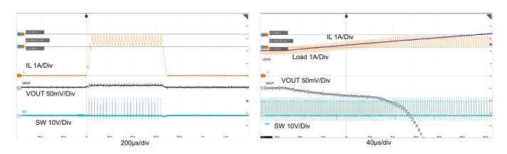
Figure 26. Short Output Protection, High-Side OC Protection
