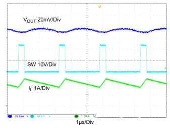
Figure 7. Stead State, 24V<sub>IN</sub>, 3.3V<sub>OUT</sub>, 0A Load
