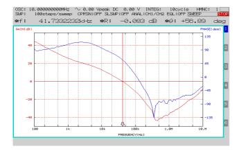
Figure 15. 24V<sub>IN</sub>, 2A, Fc = 42kHz, PM = 57° at 25°C
