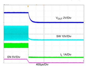
Figure 10. Output Voltage Shutdown by EN, 24V<sub>IN</sub>, 3.3V<sub>OUT</sub>, 2A
