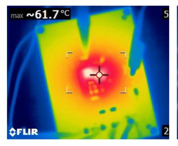
Figure 23. Thermal Image  $75V_{IN}$ ,  $12V_{OUT}$ , 500kHz, 2A, L = 15uH, HTSSOP Package, IC Temperature at  $61.7^{\circ}$ C
