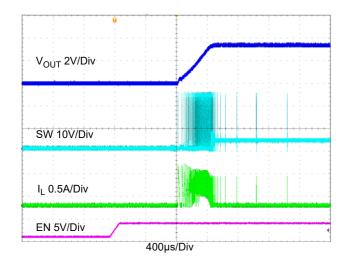
Figure 9. Output Voltage Start-Up by EN,  $24V_{\rm IN}$ ,  $3.3V_{\rm OUT}$ , 0A
