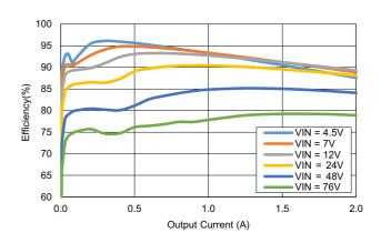
Figure 5. Efficiency vs Load, 3.3V<sub>OUT</sub>, 400kHz, QFN
