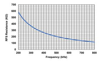
Figure 25. Switching Frequency versus FS Resistance
