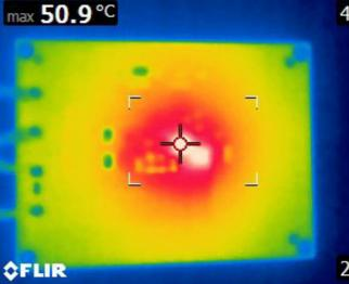
Figure 24. Thermal Image 48V<sub>IN</sub>, 3.3V<sub>OUT</sub>, 400kHz, 2A QFN Package, IC Temperature at 50.9°C
