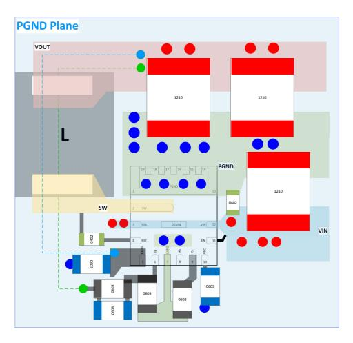
Figure 29. QFN Package Layout Recommendation
