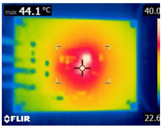
Figure 22. Thermal Image 48V<sub>IN</sub>, 3.3V<sub>OUT</sub>, 400kHz, 2A HTSSOP Package, IC Temperature at 44.1°C
