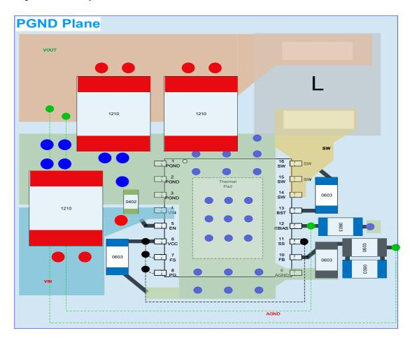
Figure 28. HTSSOP Package Layout Recommendation
