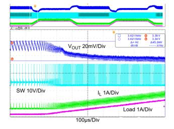
Figure 13. DCM to CCM Transition, 24V $_{\rm IN}$ , 3.3V $_{\rm OUT}$
