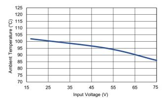
Figure 20. Derating Curve: 12V<sub>OUT</sub>, 500kHz, L=15uH, 2A, HTSSOP Package
