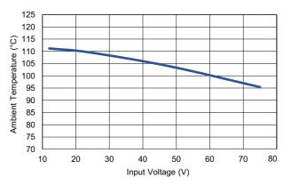
Figure 18. Derating Curve: 3.3V<sub>OUT</sub>, 400kHz, 2A, HTSSOP Package
