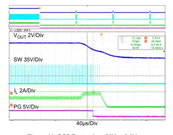
Figure 11. OCP Protection,  $76V_{IN}$ ,  $3.3V_{OUT}$
