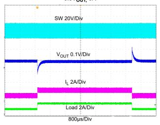
Figure 14. Load Transient,  $24V_{IN}$ ,  $3.3V_{OUT}$ , 1A to 2A to 1A
