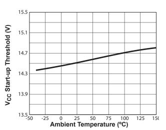
Figure 8.2 :  $V_{\text{CC}}$  Start-up Threshold vs. Temperature
