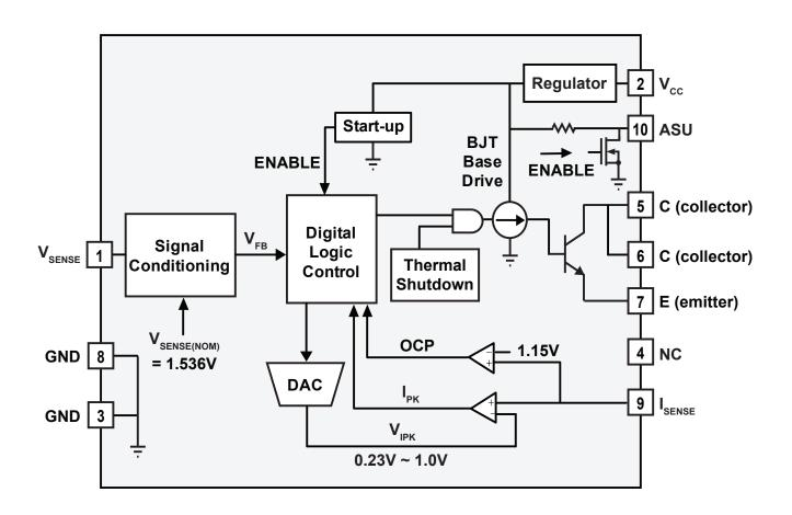
Figure 9.1 : iW1819 Functional Block Diagram
