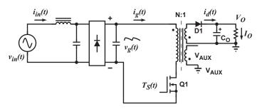
Figure 10.2 : Simplified Flyback Converter
