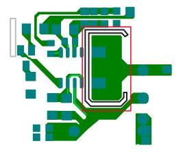
Figure 10.6 : Creepage Layout Example
