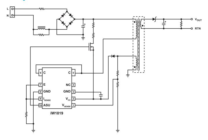
Figure 3.1: iW1819 Typical Application Circuit
