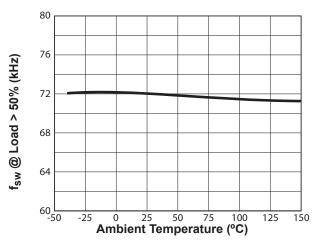
Figure 8.3 : Switching Frequency vs. Temperature<sup>1</sup>
