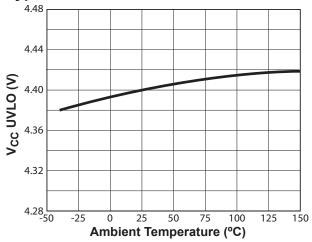
Figure 8.1 : V<sub>CC</sub> UVLO vs. Temperature
