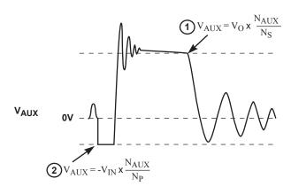
Figure 10.3: Auxiliary Voltage Waveforms
