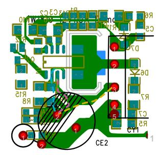
Figure 10.11a: IC and Transformer Ground Path
