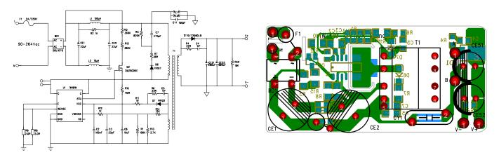
Figure 10.6a: Application Schematic of Typical iW1819 Circuit Figure 10.6b: Typical Layout of iW1819 Application Circuit
