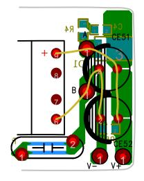
Figure 10.9a: Secondary-Side Power Path
