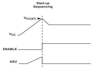
Figure 10.1: Start-up Sequencing Diagram
