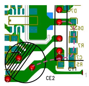
Figure 10.12a: Snubber Circuit Path
