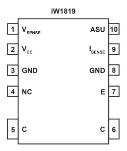
Figure 4.1: 10-Lead SOIC Batwing Package
