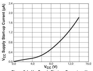
Figure 8.4 :  $V_{\text{CC}}$  Supply Start-up Current vs.  $V_{\text{CC}}$
