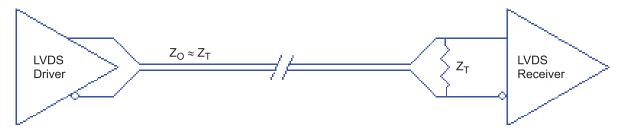
Figure 3A. Standard LVDS Termination
