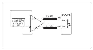
1.8V LVDS Output Load Test Circuit
