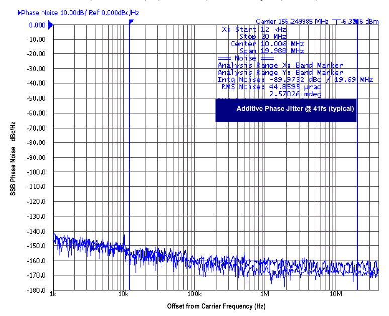
As with most timing specifications, phase noise measurements have issues relating to the limitations of the measurement equipment. The noise floor of the equipment can be higher or lower than the noise floor of the device. Additive phase noise is dependent on both the noise floor of the input source and measurement equipment.
