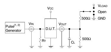
Test Circuits for All Outputs
