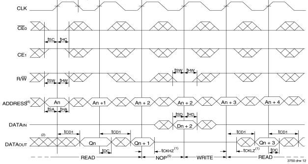
Timing Waveform of Flow-Through Read-to-Write-to-Read (**OE** Controlled)<sup>(3)</sup>
