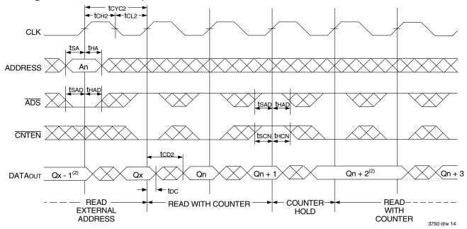
Timing Waveform of Flow-Through Counter Read with  ${\rm Address\,Counter\,Advance}^{(1)}$
