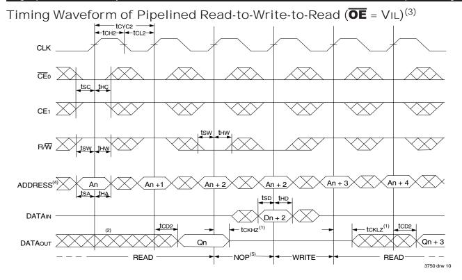
Timing Waveform of Pipelined Read-to-Write-to-Read (**OE** Controlled)(3)
