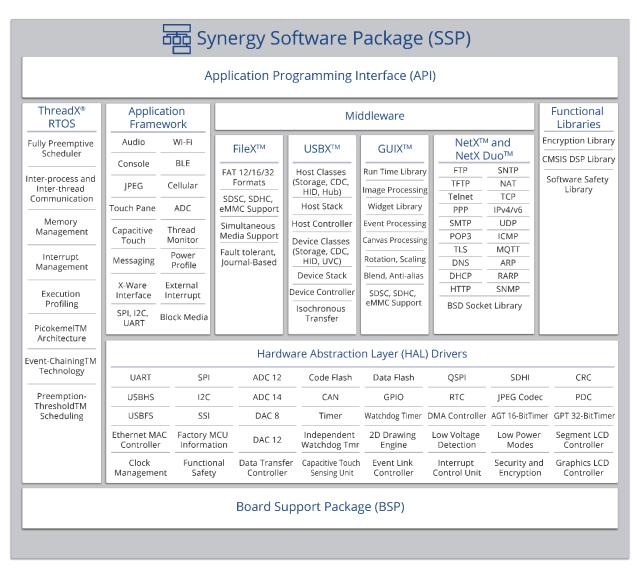
Figure 7: Synergy Software Package
