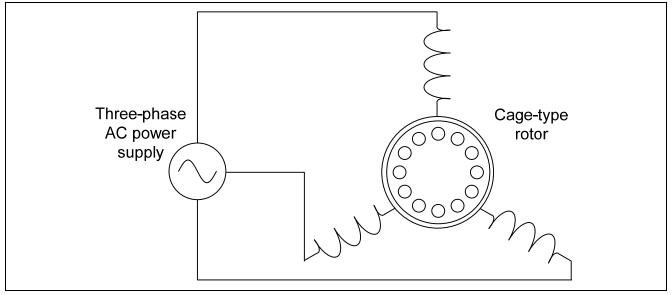
Figure 2-1 Configuration Diagram of A Three-phase Induction Motor
