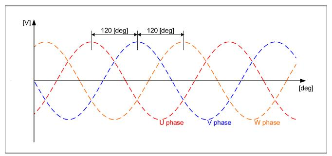
Figure 2-3 Three-phase Voltage Waveforms with 120-degree Phase Differences
