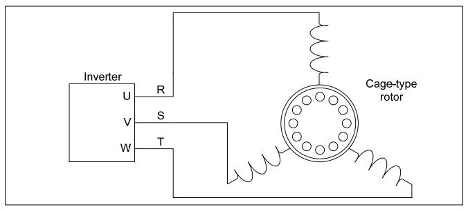
Figure 2-2 Configuration Diagram of Inverter Drive
