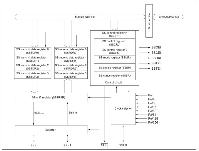
Figure 2 Block Diagram of the SSU Module
