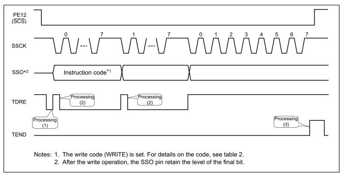
Figure 4 Processing to Write Data
