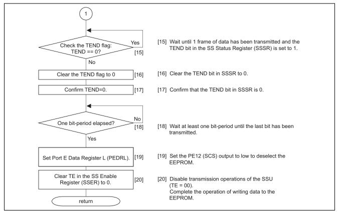
Figure 8 Processing for EEPROM-Data Reading (2)
