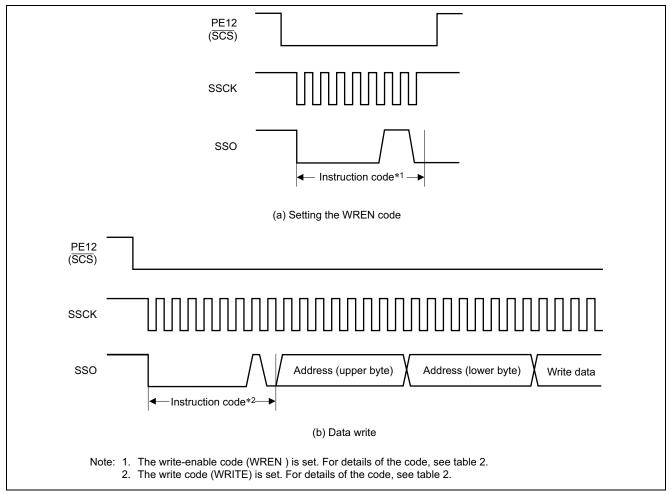
Figure 3 Details of Transfer to Write Data from the EEPROM
