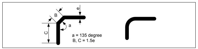
Figure 3 Wiring Corner Angle
