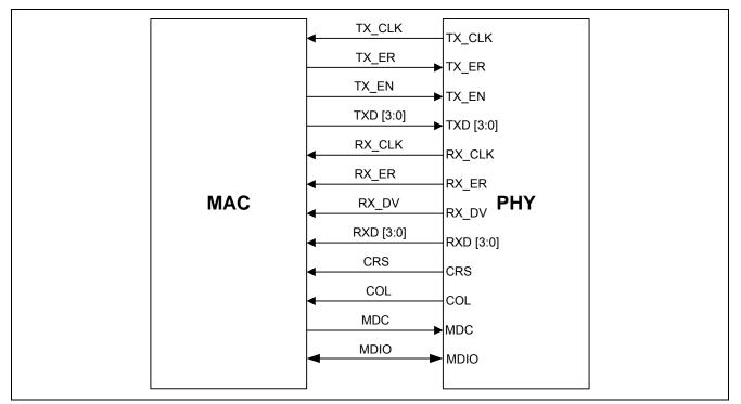
Figure 1 MII Signal Connection
