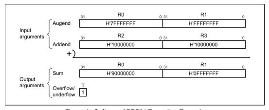
Figure 1 Software ADDS64 Execution Example
