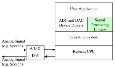
Figure 1. User System Block Diagram
