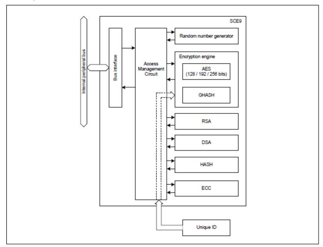
Figure 1. SCE9 Structural Features
