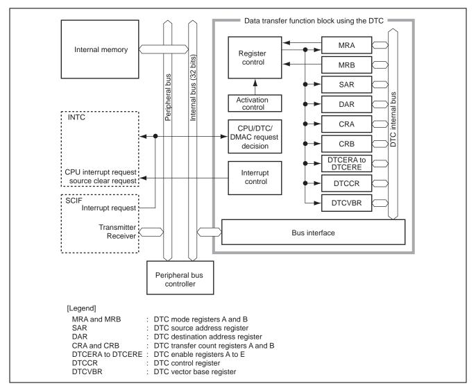
Figure 3 Block Diagram of DTC Used for Data Transfer
