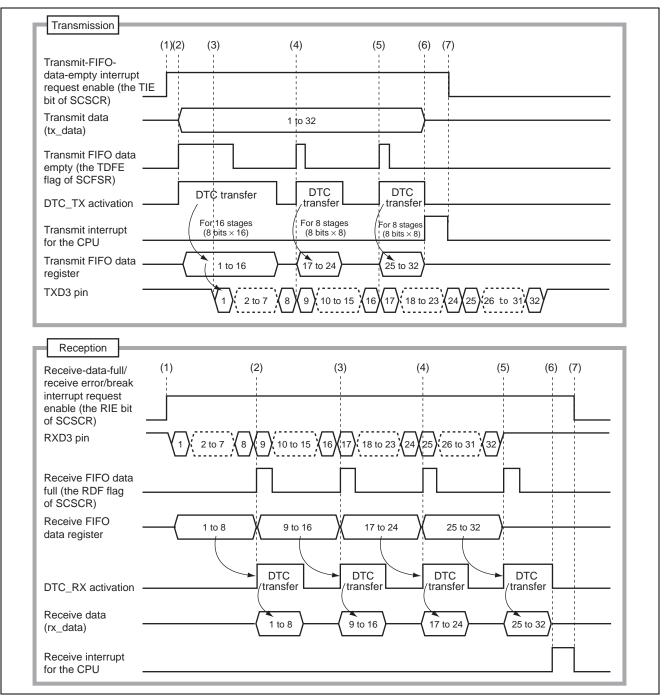
Figure 4 Principles of Operation
