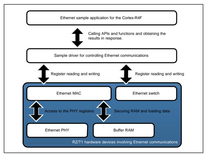
Figure 6.1 Block Diagram of Ethernet Application Software
