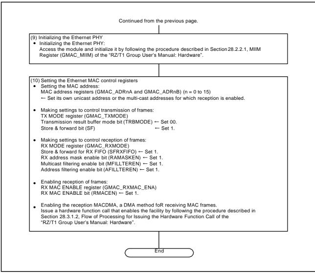
Figure 5.5 Flow of Initialization of the Ethernet MAC (5)
