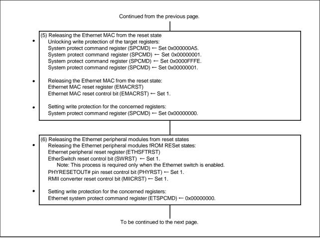
Figure 5.3 Flow of Initialization of the Ethernet MAC (3)
