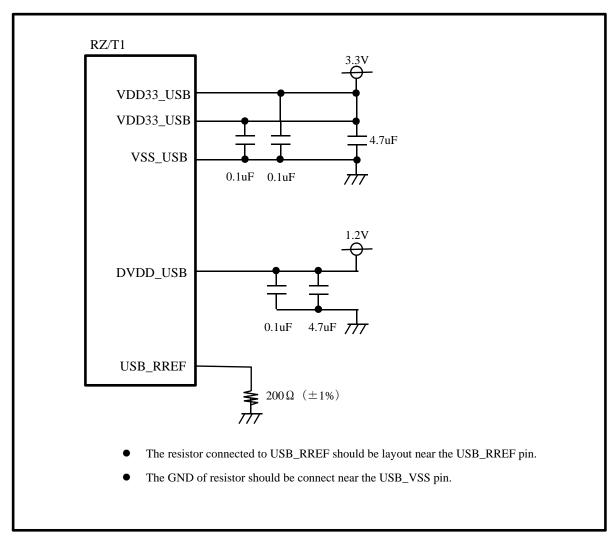
Figure 3 Example of Decoupling Capacitor Allocation
