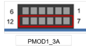
Figure 47: Connection Pmod LED module to RZ/G2L or RZ/G3S
