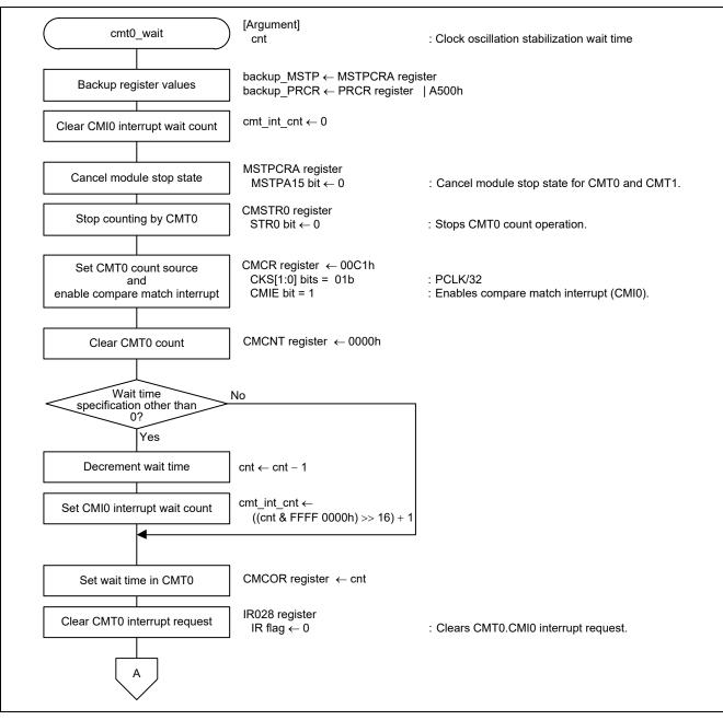
Figure 3.13 Software Wait Cycles Using CMT0 (1/2)
