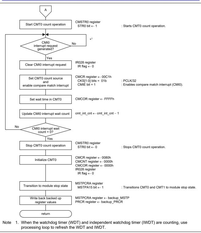
Figure 3.14 Software Wait Cycles Using CMT0 (2/2)
