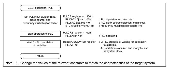
Figure 3.8 PLL Clock Oscillation Enable
