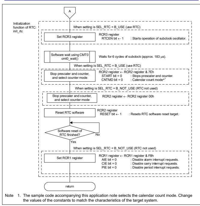
Figure 3.11 Sub-clock Oscillation Enable (2/2)
