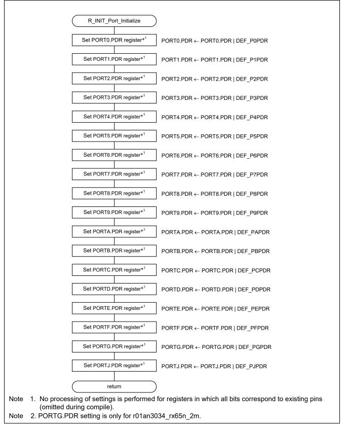
Figure 3.3 Initial Nonexistent Port Settings
