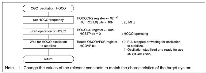
Figure 3.9 HOCO Clock Oscillation Enable
