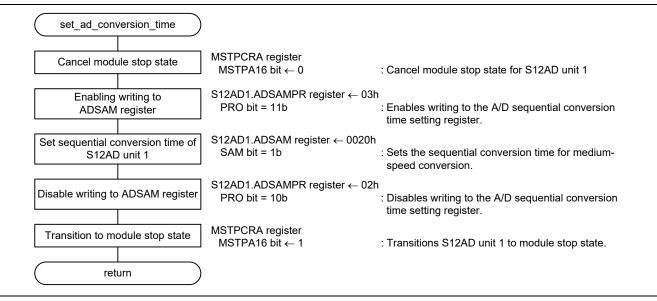
Figure 3.15 A/D Sequential Conversion Time Settings
