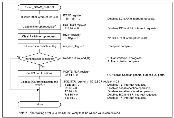
Figure 5.10 DMAC0 Transfer Complete Interrupt Handler
