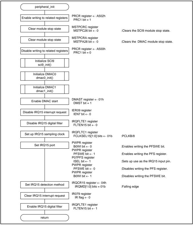
Figure 5.5 Peripheral Function Initialization
