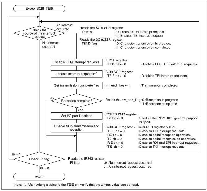
Figure 5.12 SCI9 Transmission Complete Interrupt Handler
