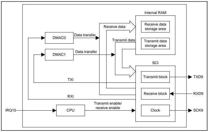
Figure 1.1 Block Diagram
