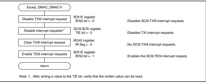
Figure 5.11 DMAC1 Transfer Complete Interrupt Handler
