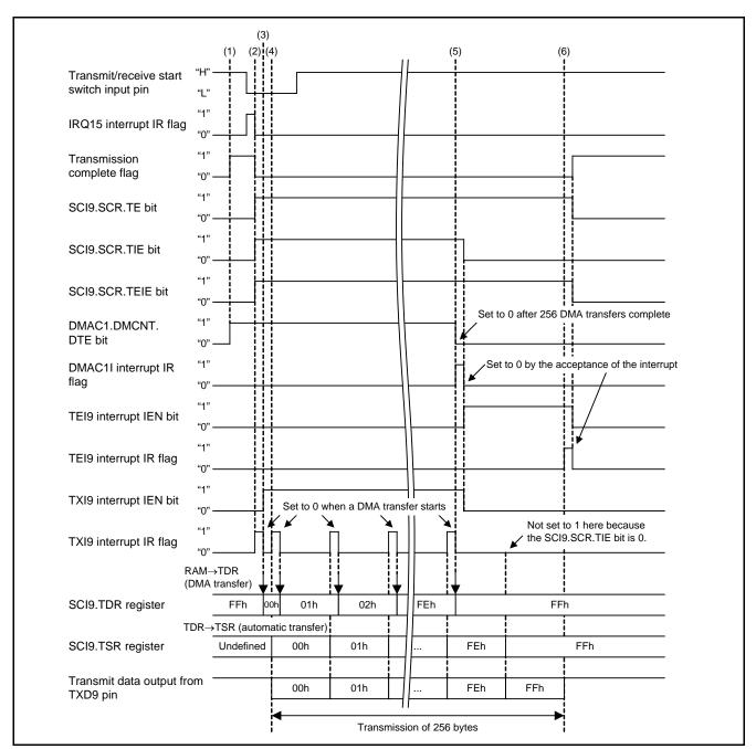
Figure 5.1 Transmission Operation Timing Chart
