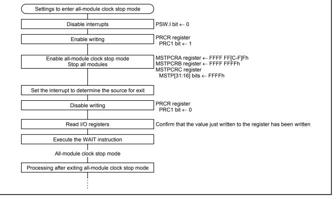
Figure 3.2 Procedure to Enter All-Module Clock Stop Mode
