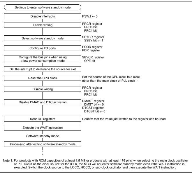
Figure 3.3 Procedure to Enter Software Standby Mode
