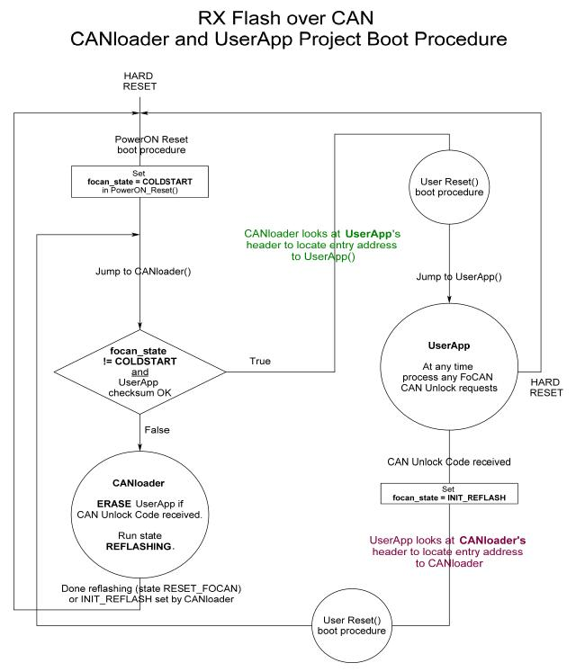
Figure 7. Flash over CAN boot procedure; how the common variable 'focan\_state' is used.
