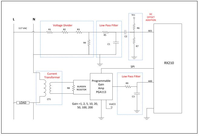
Figure 5 Analog Front End for RX210 based Energy Meter
