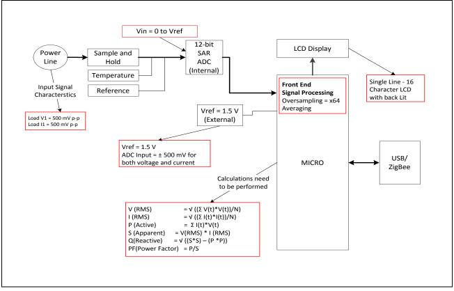
Figure 2 Signal Flow Diagram of Energy Meter
