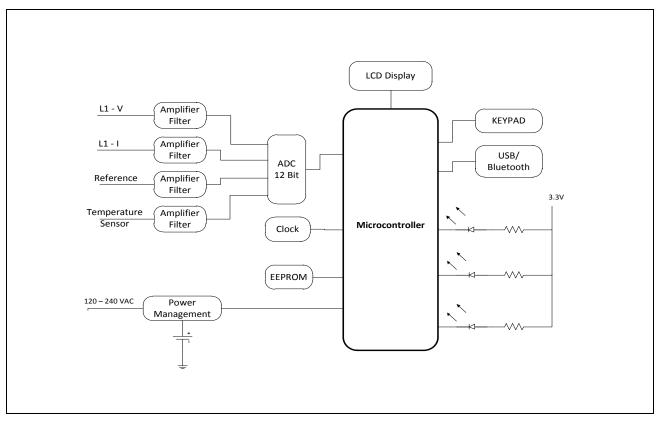
Figure 1 Block Diagram Energy Meter
