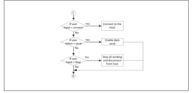
Figure 9 Communication Software Flow Chart
