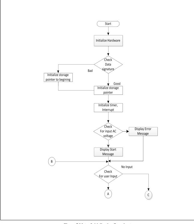
Figure 7 Meter Initialization flow chart
