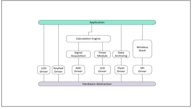
Figure 6 Software Architecture of Energy Meter
