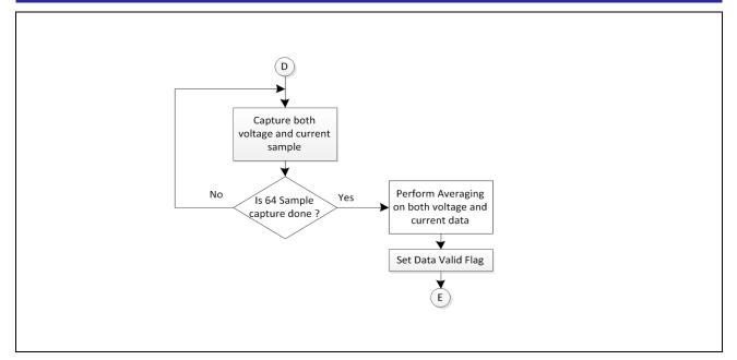
Figure 10 Front end signal Processing Flow chart
