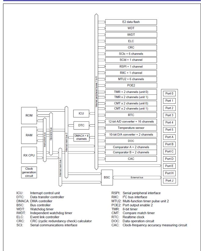
Figure 3 Block Diagram of RX210
