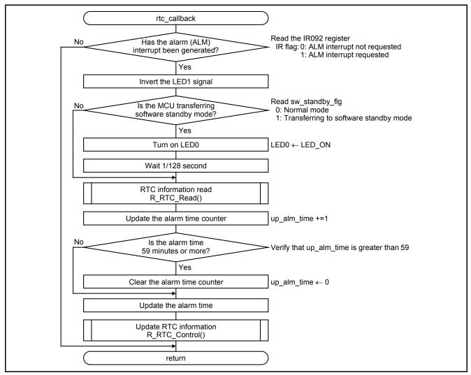
Figure 5.7 Alarm (ALM) Interrupt Handling
