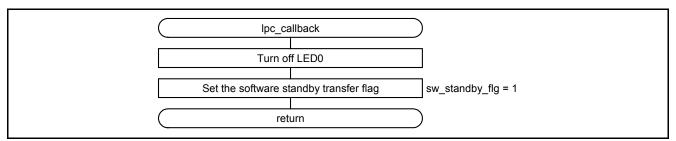
Figure 5.8 Processing Before Entering Software Standby Mode
