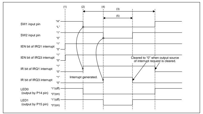
Figure 5.1 Timing Chart Showing Occurrence of Multiple Interrupts
