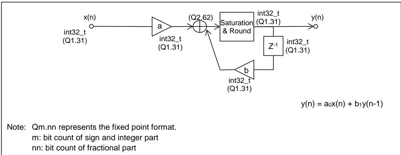
Figure 1 Signal Flow Chart of Single-pole IIR filter
