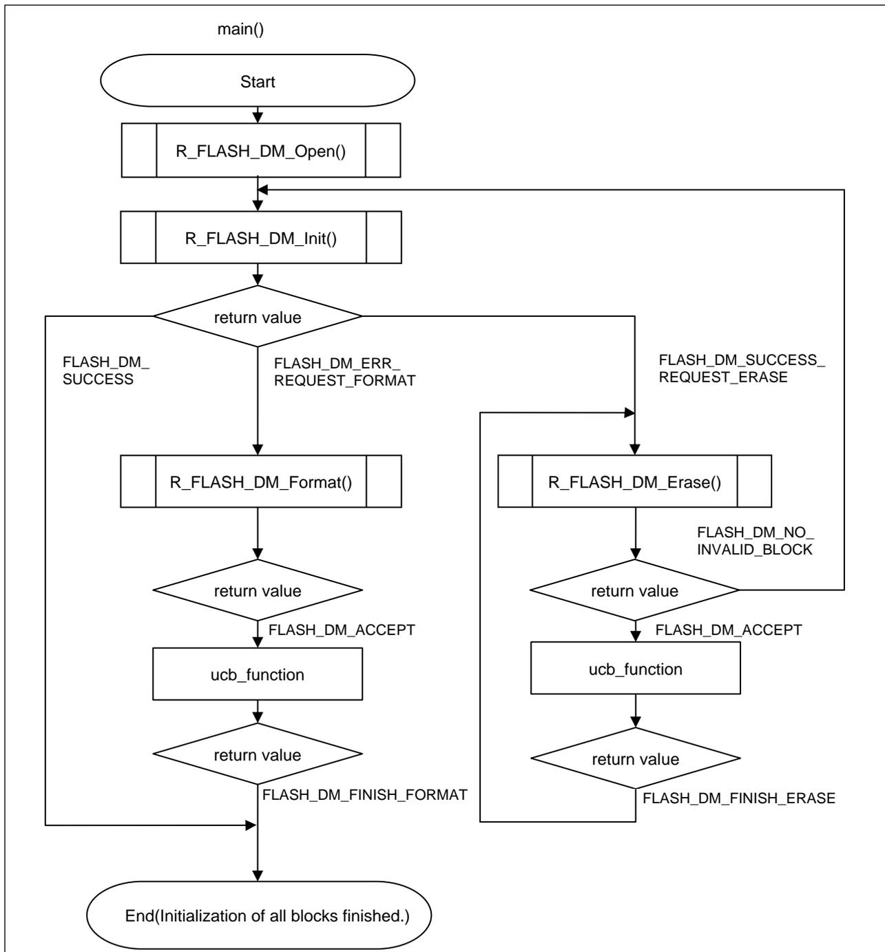
Figure 1.3 Example of processing after R\_FLASH\_DM\_Init() (Flash Type 1)
