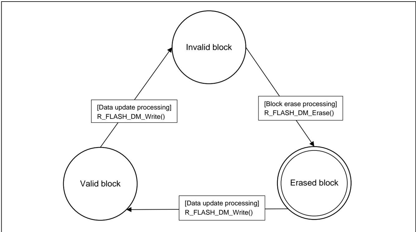
**Figure 5.3 Block States (Flash Types 3, 4, and 5)**
