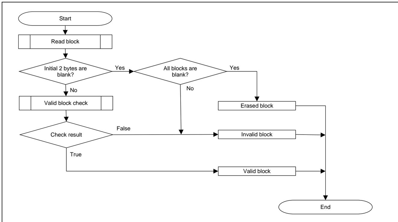
**Figure 5.4 Block State Determination Flowchart (Flash Types 3, 4, and 5)**
