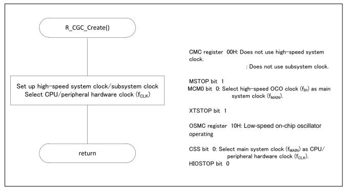
Figure 4.4 CPU Clock Setup
