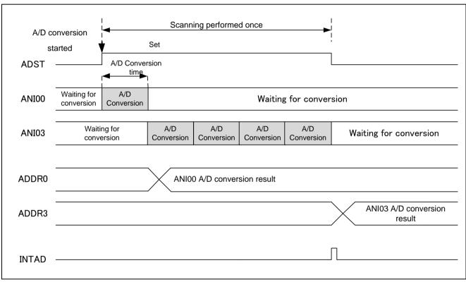
Figure 1.1 Outline of the A/D Converter Conversion Processing
