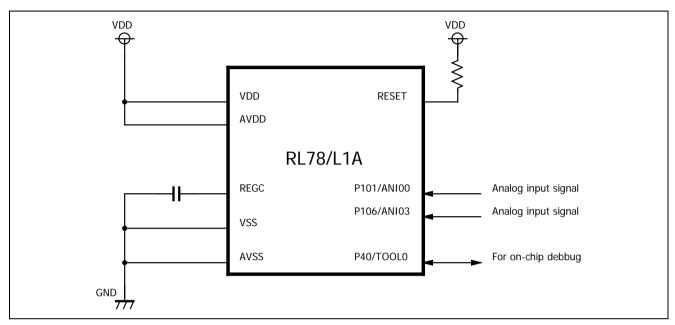
**Figure 3.1 Hardware Configuration**
