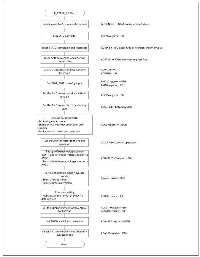
Figure 4.5 A/D Converter Setup
