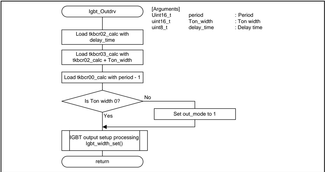
Figure 4.14 IGBT Output Driver Setup
