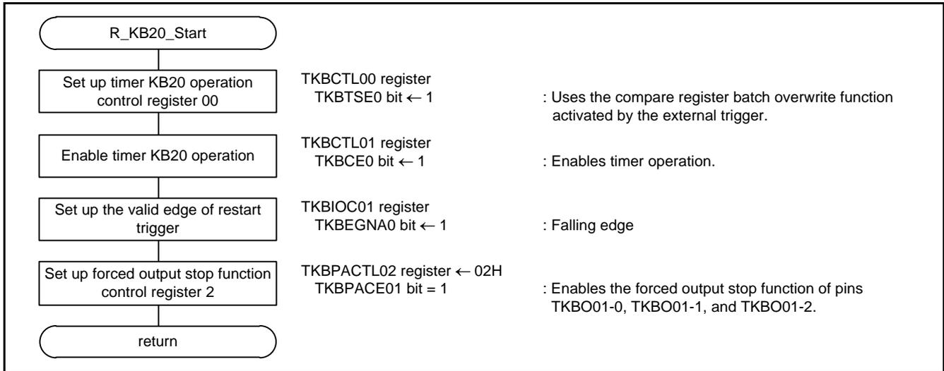
Figure 4.12 Enable Timer KB20 Operation
