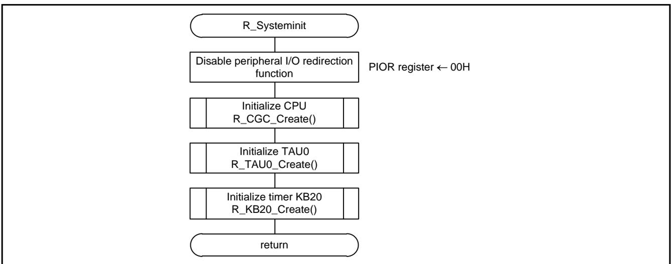
Figure 4.4 Peripheral Function Initialization
