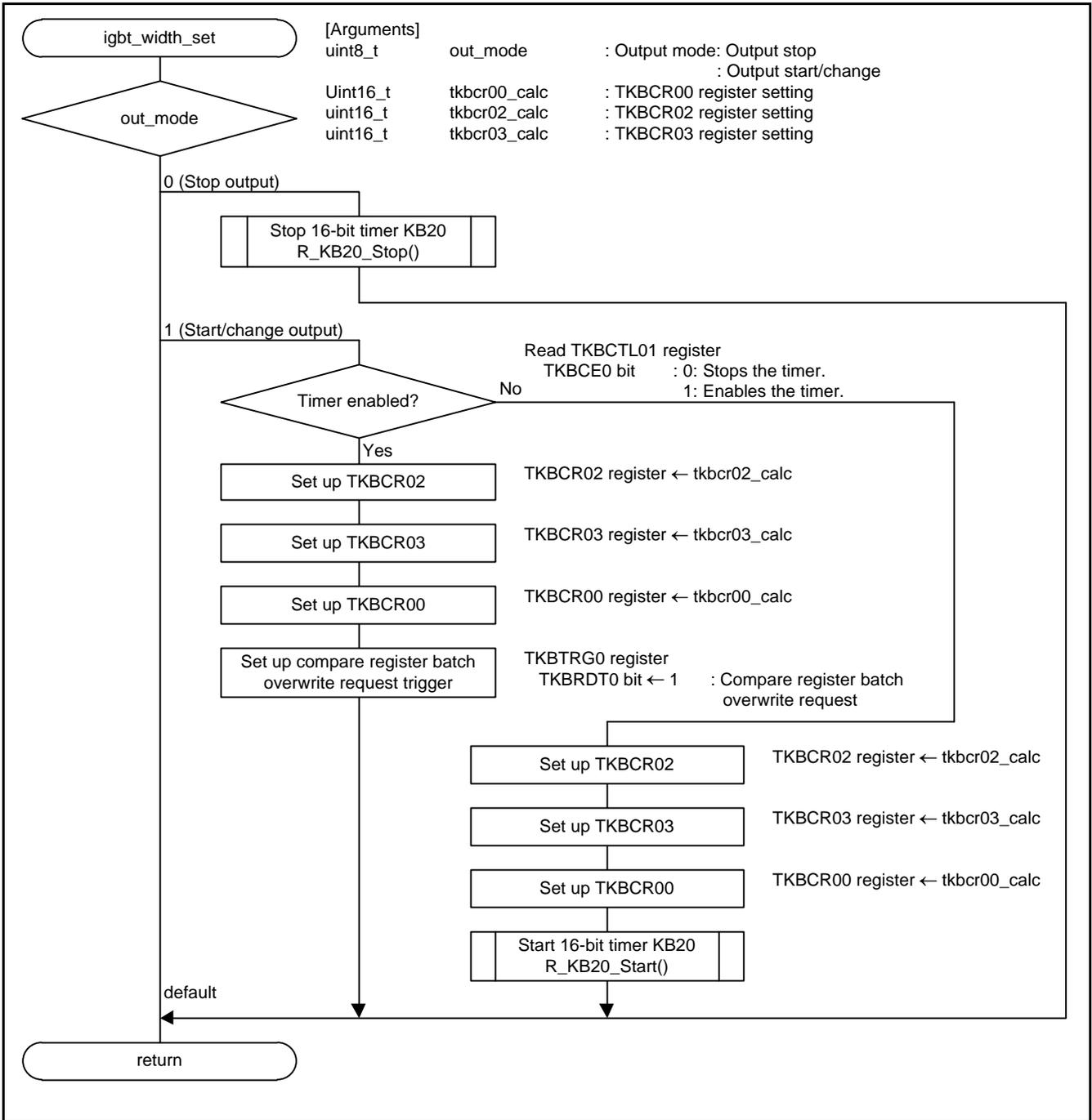
Figure 4.15 IGBT Output Setup
