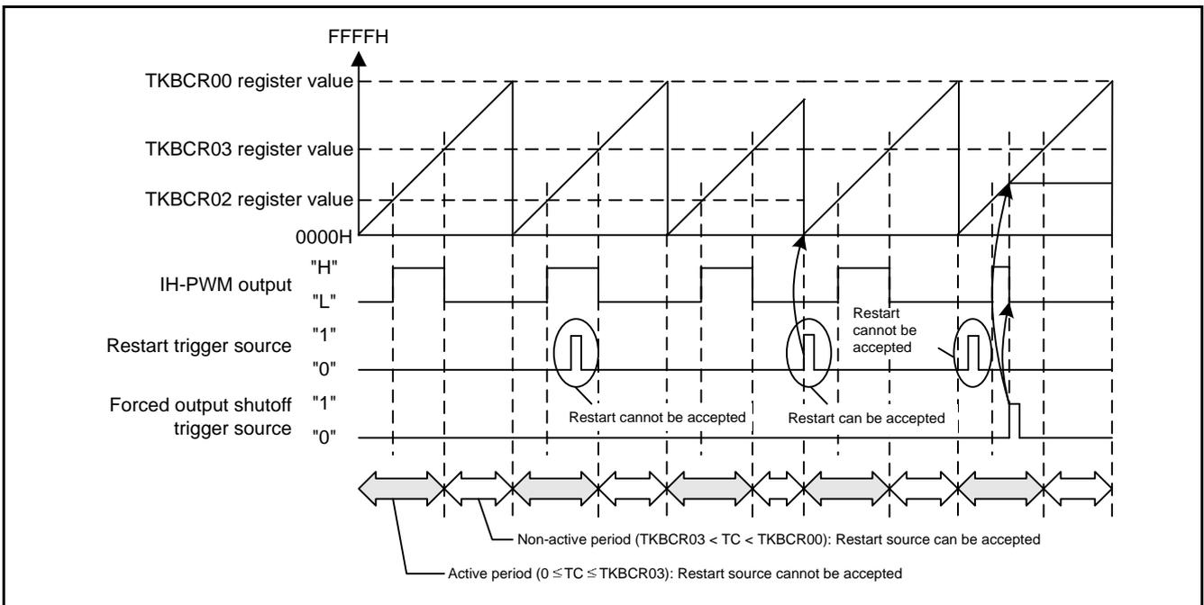
**Figure 1.1 PWM Output Function for IH Control**
