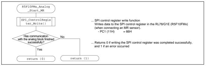
Figure 6.11 Flowchart for R5F10FMx\_Analog\_Start\_MR Function
