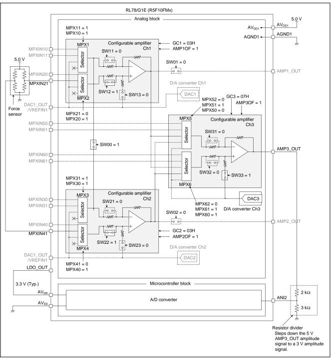
Figure 5.3 Connection Between Configurable Amplifier Channels Ch1 to Ch3 and Force Sensor, and Between Configurable Amplifier Channels Ch1 to Ch3 and A/D Converter
