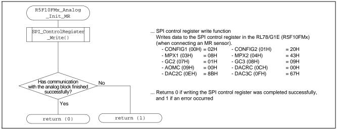
Figure 6.9 Flowchart for R5F10FMx\_Analog\_Init\_MR Function
