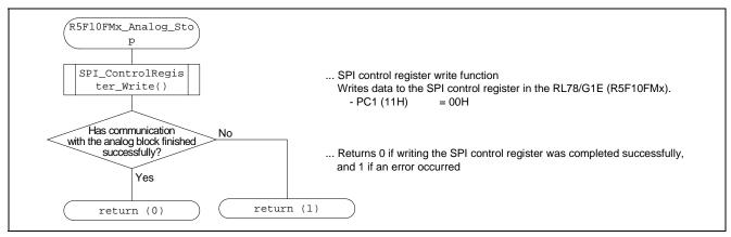
Figure 6.13 Flowchart for R5F10FMx\_Analog\_Stop Function
