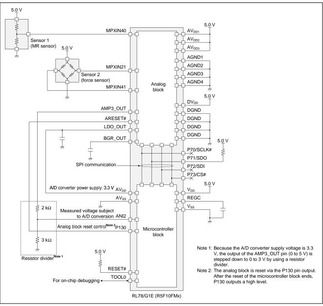
Figure 4.1 Hardware Configuration
