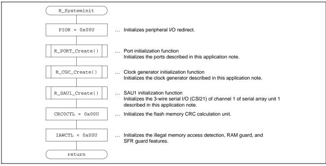
Figure 6.4 Flowchart for R\_Systeminit Function
