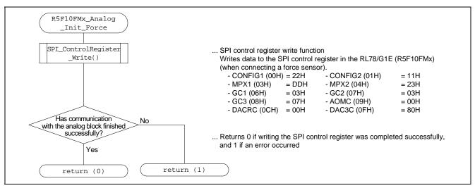
Figure 6.10 Flowchart for R5F10FMx\_Analog\_Init\_Force Function
