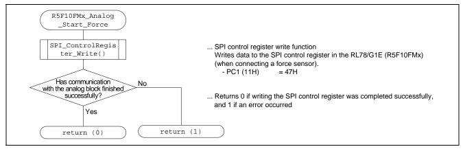
Figure 6.12 Flowchart for R5F10FMx\_Analog\_Start\_Force Function
