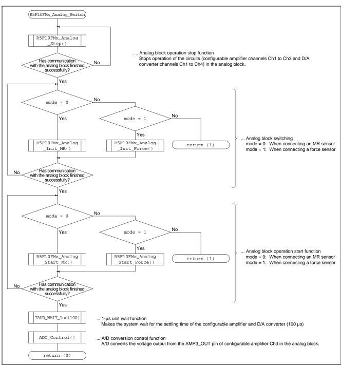
Figure 6.8 Flowchart for R5F10FMx\_Analog\_Switch Function
