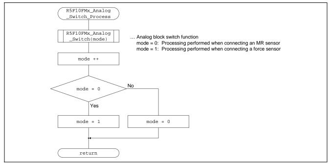
Figure 6.7 Flowchart for R5F10FMx\_Analog\_Switch\_Process Function
