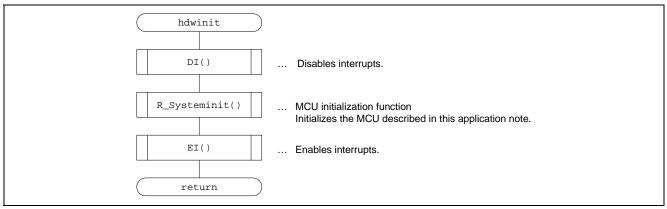
Figure 6.3 Flowchart for hdwinit Function
