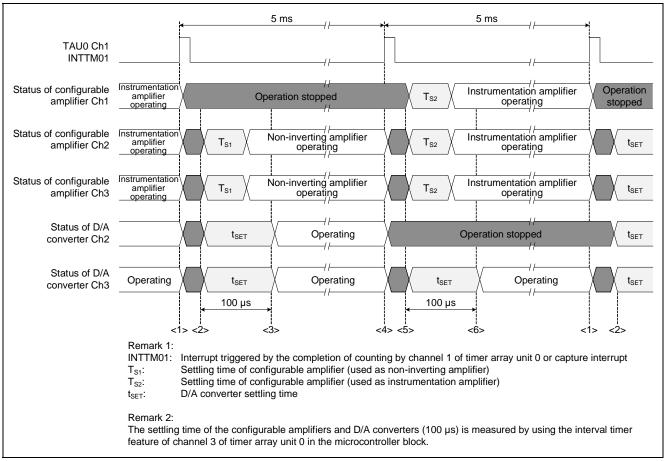
Figure 6.1 Timing of Amplifier Reconfiguration in Analog Block
