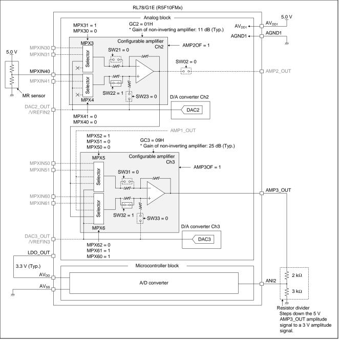
Figure 5.2 Connection Between Configurable Amplifier Channels Ch2 and Ch3 and MR Sensor, and Between Configurable Amplifier Channels Ch2 and Ch3 and A/D Converter Follow the procedure below to start configurable amplifier Ch1 (used as a non-inverting amplifier).
