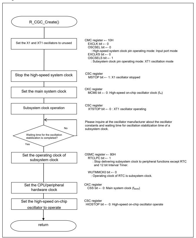
Figure 5.7 CPU Clock Initialization
