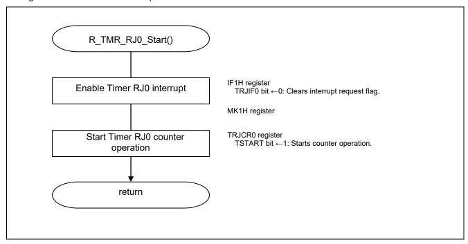
Figure 5.14 Timer RJ0 Operation Start
