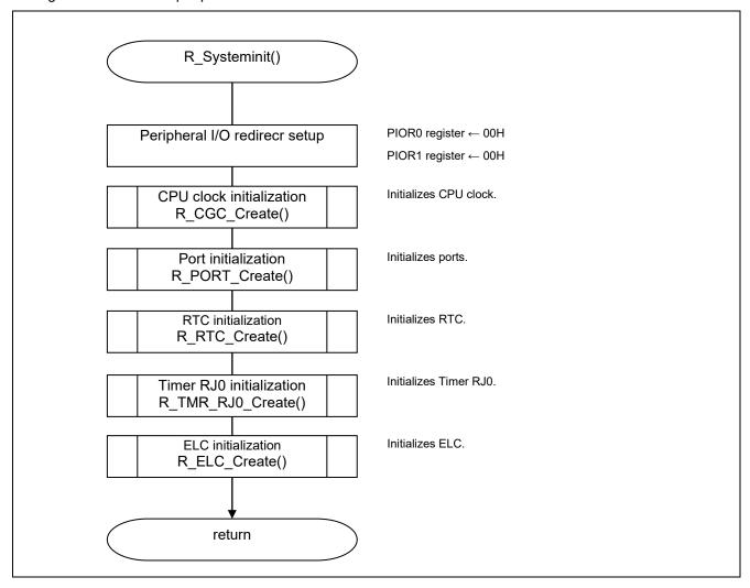
Figure 5.6 Peripheral Function Initialization
