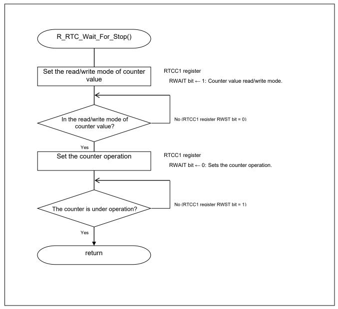
Figure 5.15 Wait Before Shifting to RTC STOP Mode
