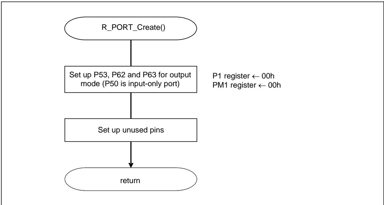
**Figure 6.5 I/O Port Setup**
