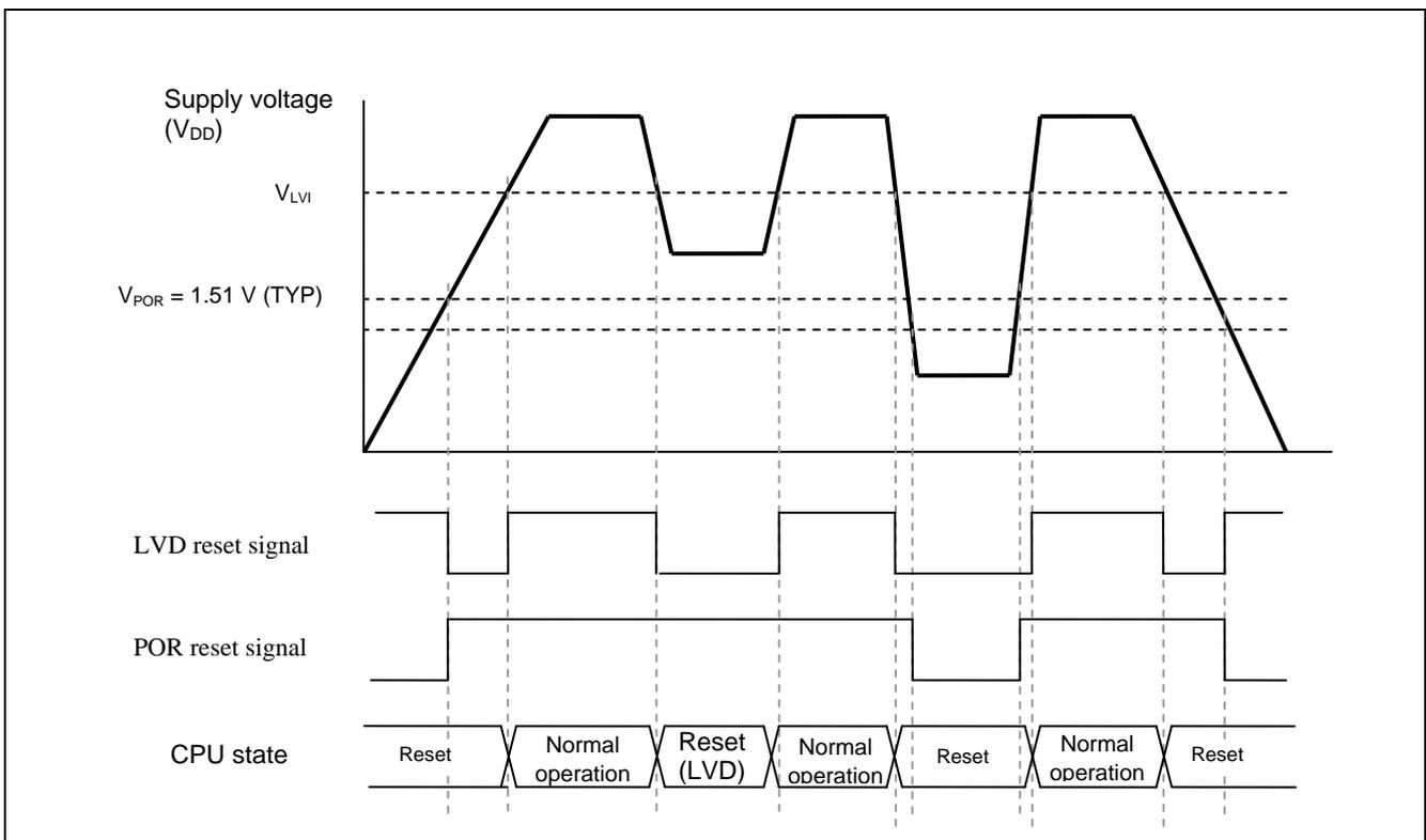
**Figure 2.1 Overview of LVD Operation (Reset Mode)**
