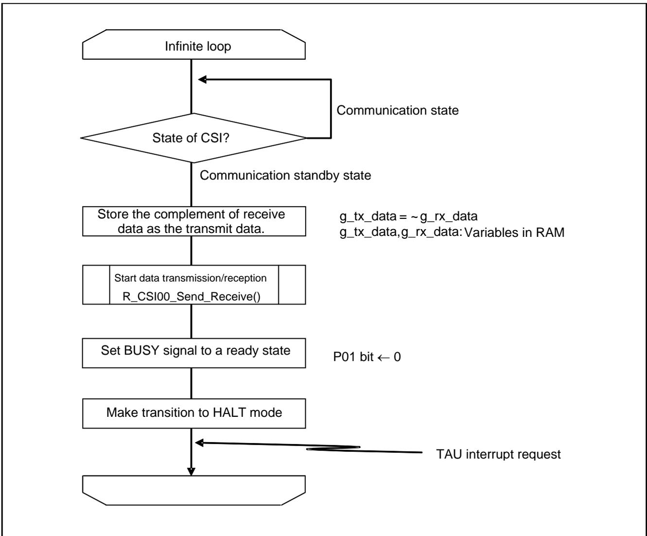
**Figure 5.11 Infinite Loop in Main Processing**
