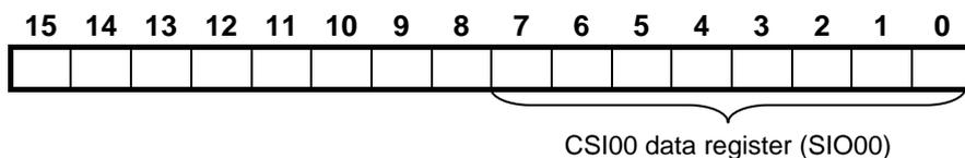
Write transmit data to the lower eight bits.
