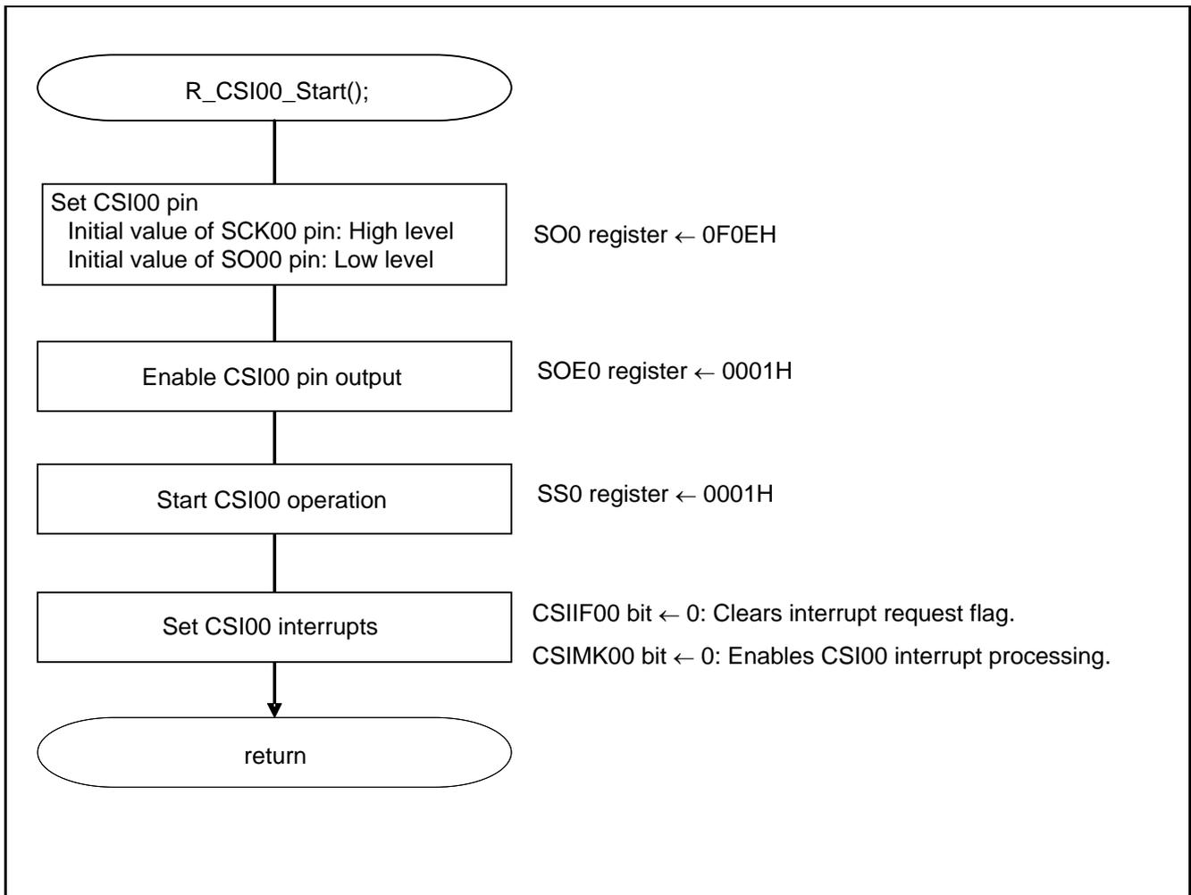
**Figure 5.10 SAU0 Channel 0 (CSI00) Operation Start Processing**
