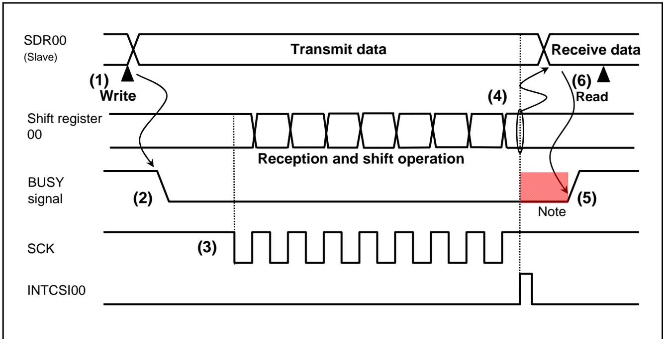
**Figure 1.2 Handshake Operation and Communication**
