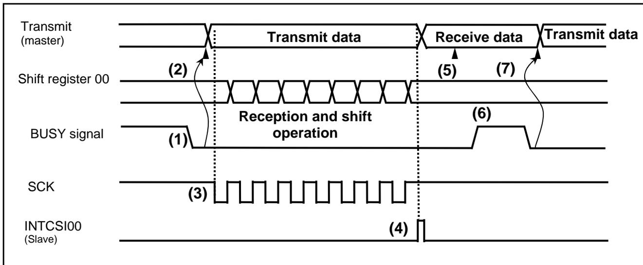
**Figure 1.4 Example of BUSY Signal Edge Detection in the Master**
