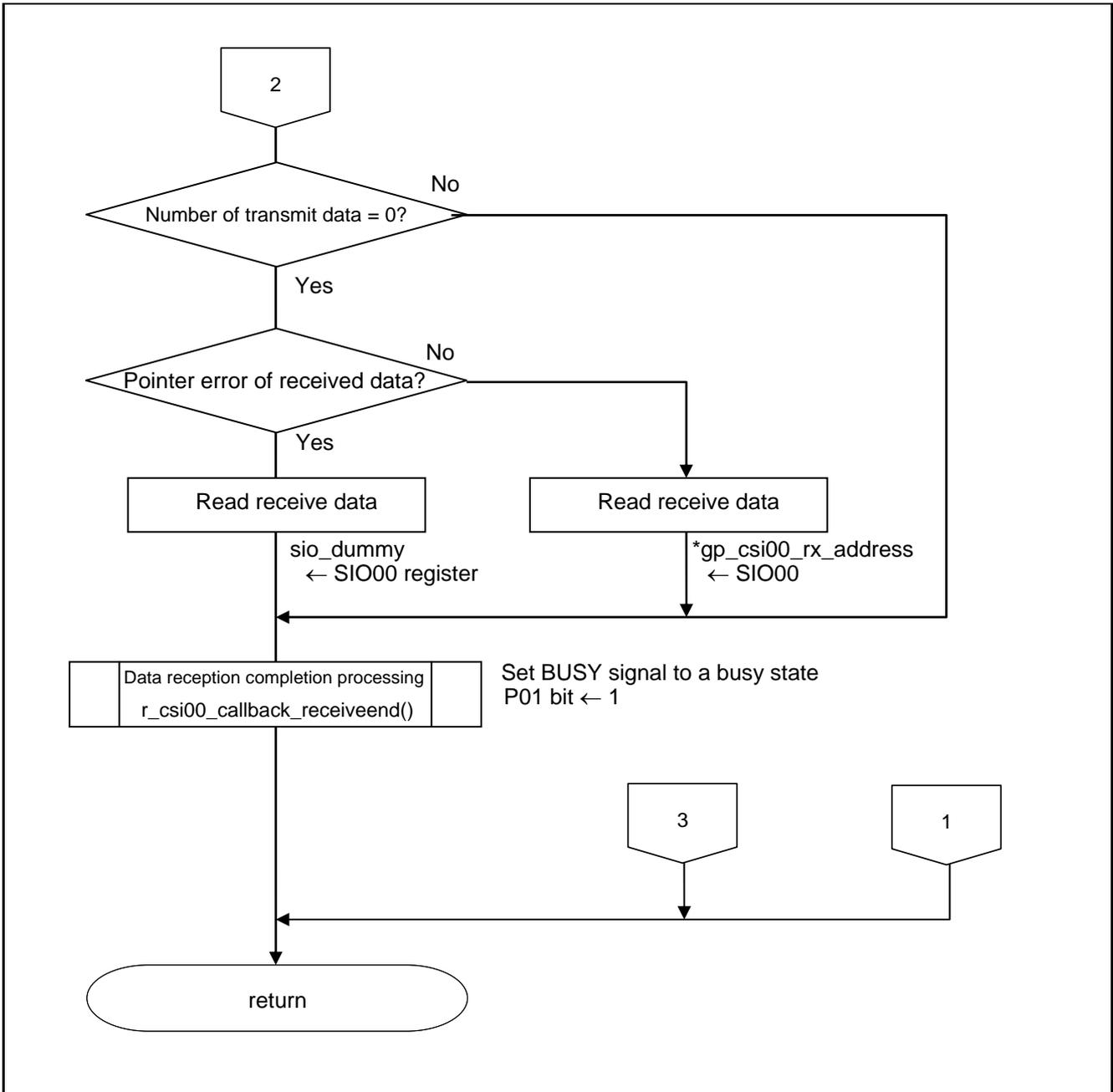
Figure 5.15 CSI00 Transfer End Interrupt Processing (2/2)
