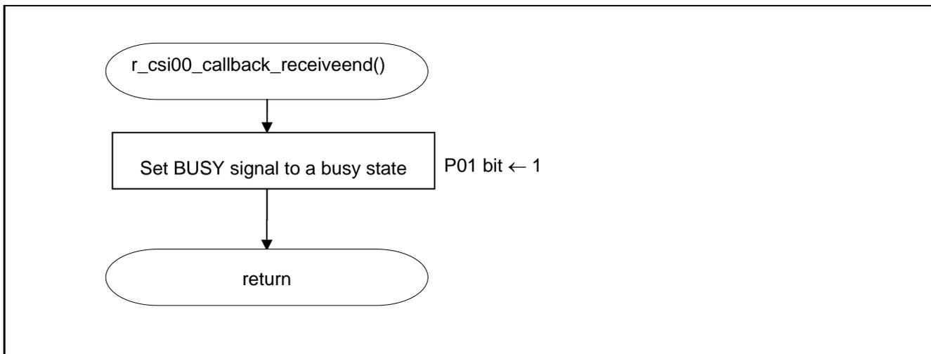
**Figure 5.16 Data reception completion processing**
