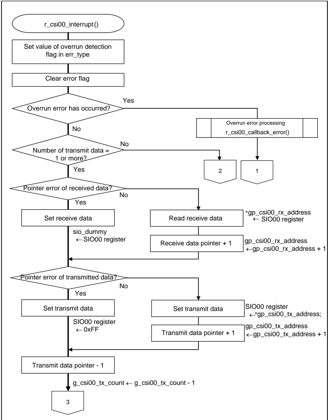
Figure 5.14 CSI00 Transfer End Interrupt Processing (1/2)
