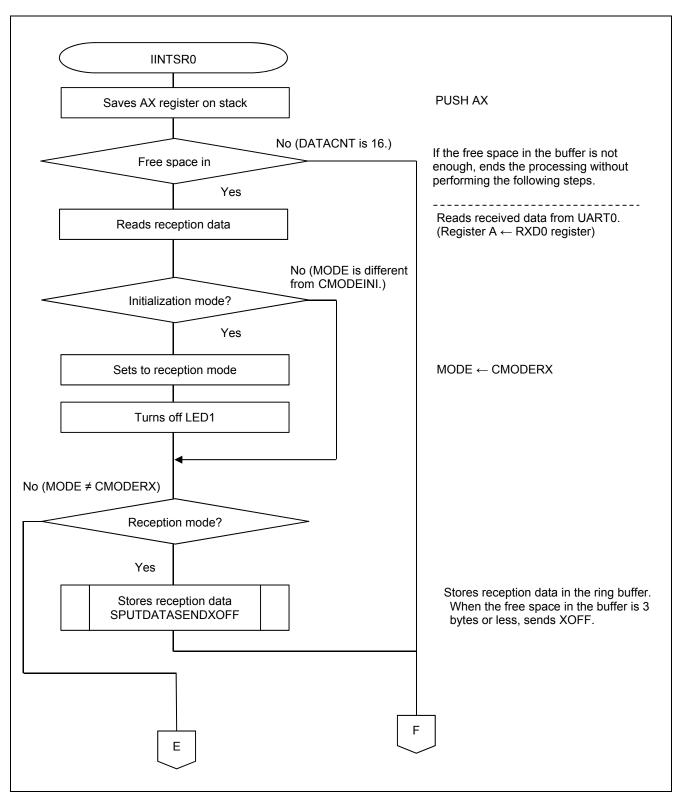
Figure 5.21 UART0 Reception End Interrupt Processing (1 of 2)
