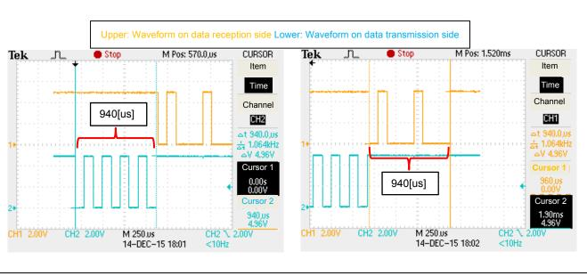
Figure 6.4 Waveforms on Data Transmission Side (Left) and Data Reception Side (Right) (9600bps)
