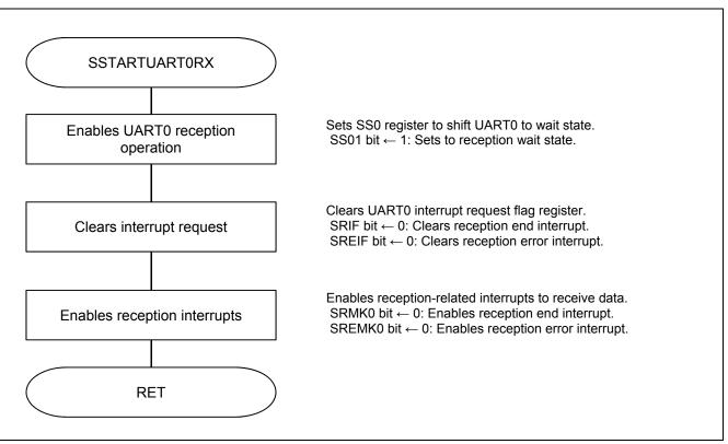
Figure 5.13 UART0 Reception Enabling Processing
