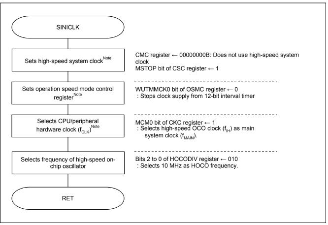
Figure 5.3 Setting of Clock Generation Circuit
