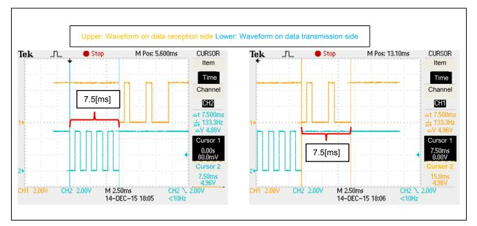
Figure 6.3 Waveforms on Data Transmission Side (Left) and Data Reception Side (Right) (1200bps)
