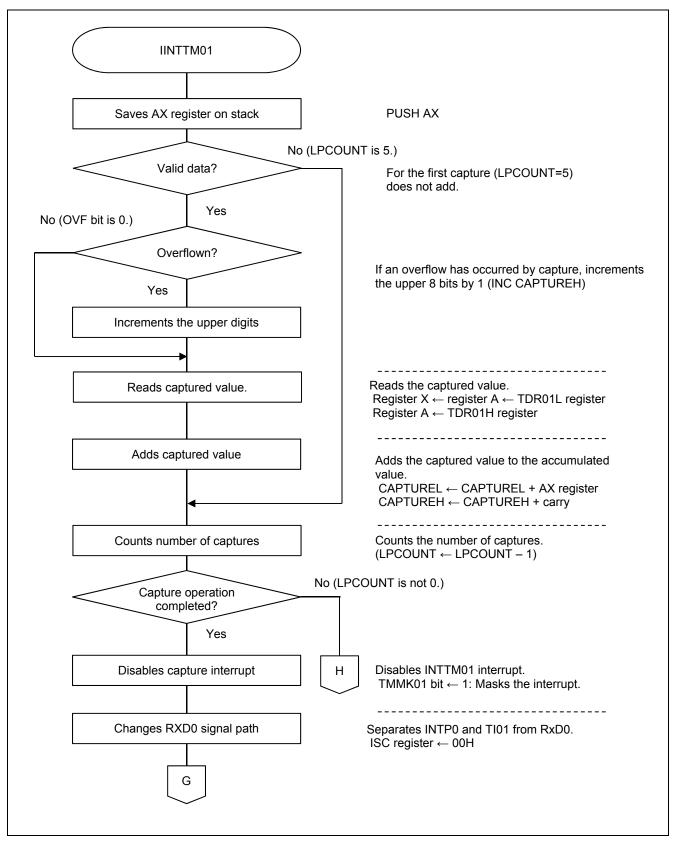
Figure 5.25 INTTM01 Interrupt Processing (1 of 2)
