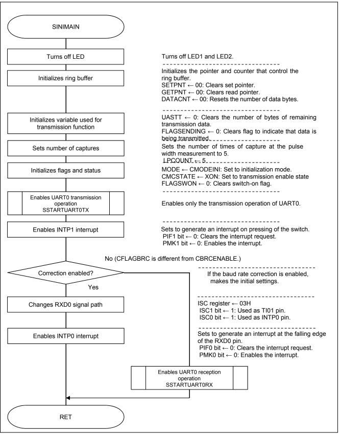
**Figure 5.10 Main Initialization Processing**
