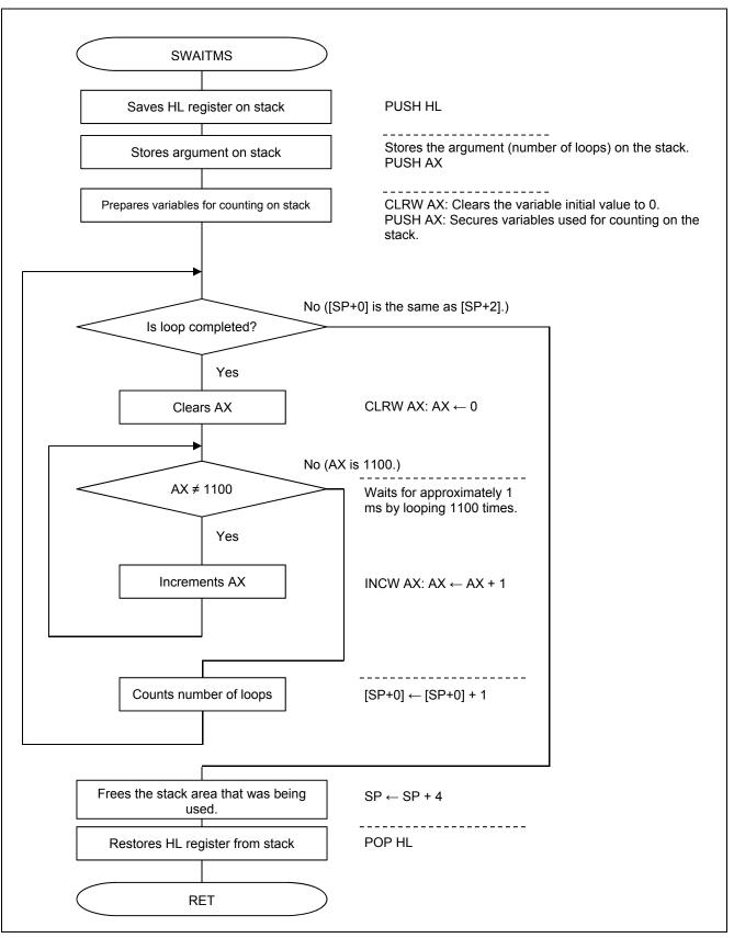
Figure 5.11 Wait Processing (millisecond units)
