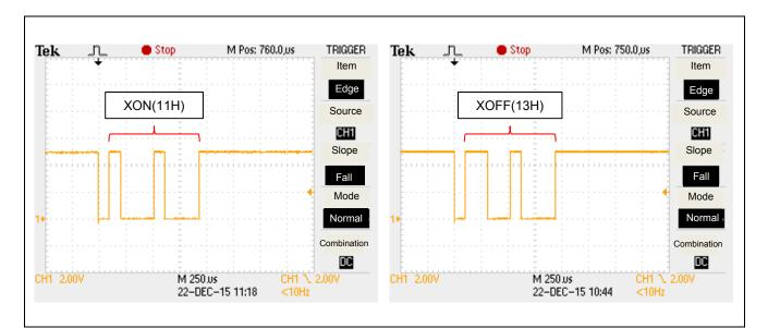
Figure 6.2 Waveforms when XON (Left) and XOFF (Right) are Transmitted
