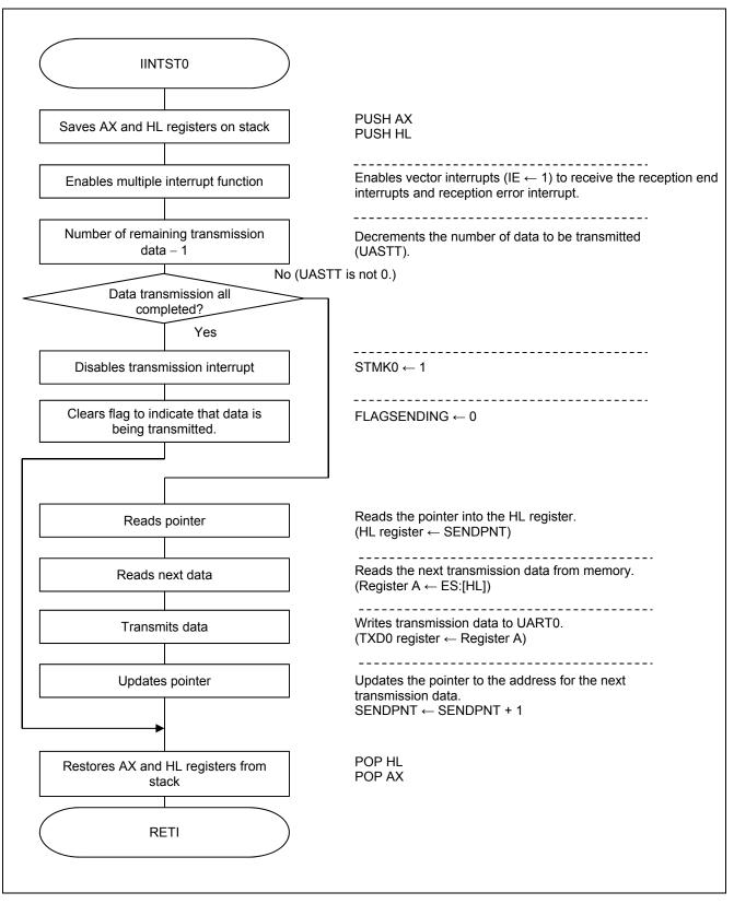
Figure 5.24 UART0 Transmission End Interrupt Processing
