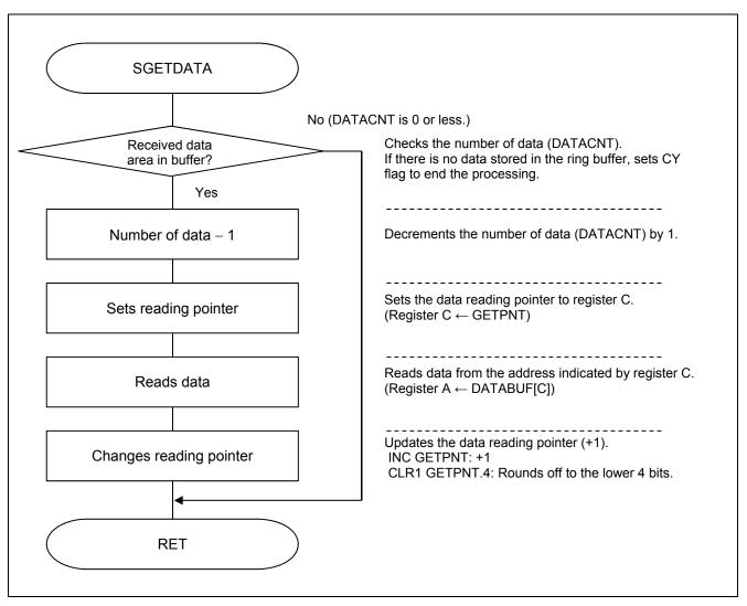
Figure 5.19 Ring Buffer Read Processing
