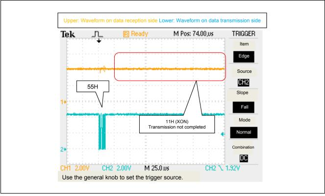
Figure 6.8 Waveform when Baud Rate Correction Fails
