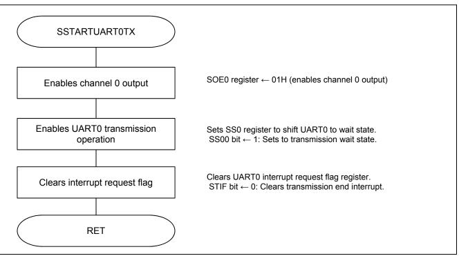
Figure 5.12 UARTO Transmission Enabling Processing
