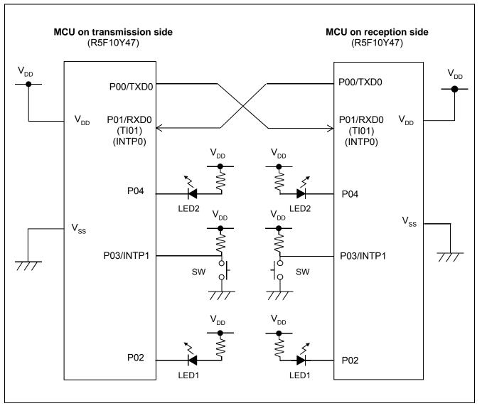
Figure 4.1 Hardware Configuration Example
