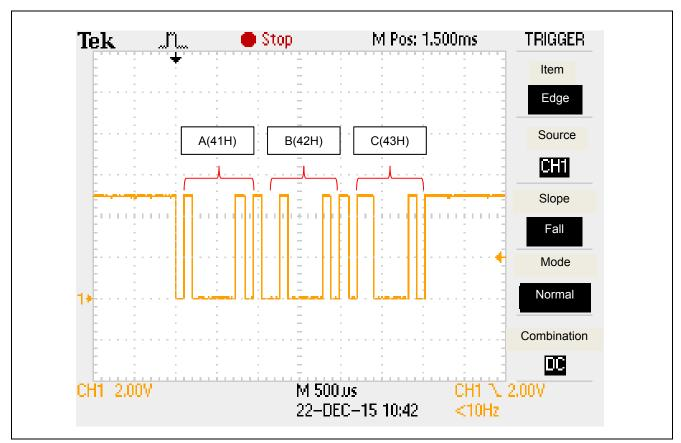
Figure 6.1 Waveform when "ABC" is Transmitted
