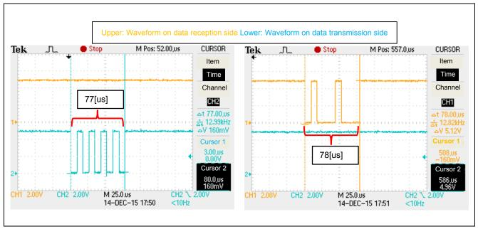
Figure 6.6 Waveforms on Data Transmission Side (Left) and Data Reception Side (Right) (115200bps)
