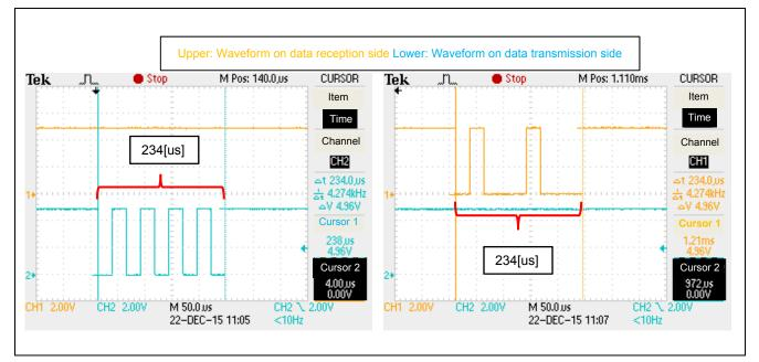
Figure 6.5 Waveforms on Data Transmission Side (Left) and Data Reception Side (Right) (38400bps)
