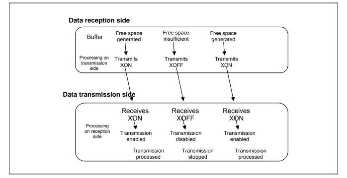
Figure 1.2 Operation of Handshake Communication Using Software
