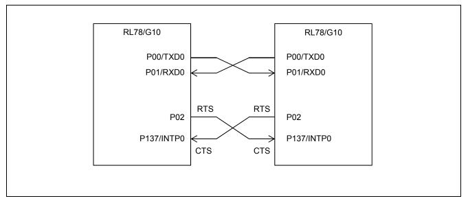
Figure 1.1 Operation of Handshake Communication using Hardware
