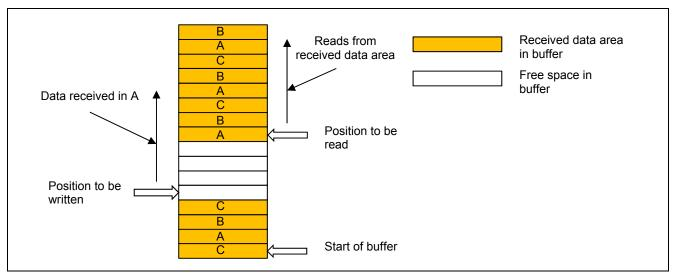
Figure 1.3 Ring Buffer Structure
