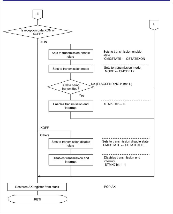
Figure 5.22 UARTO Reception End Interrupt Processing (2 of 2)
