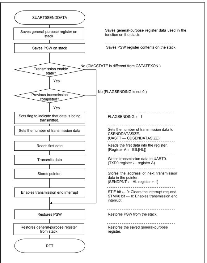
Figure 5.15 UART0 Data Transmission Processing
