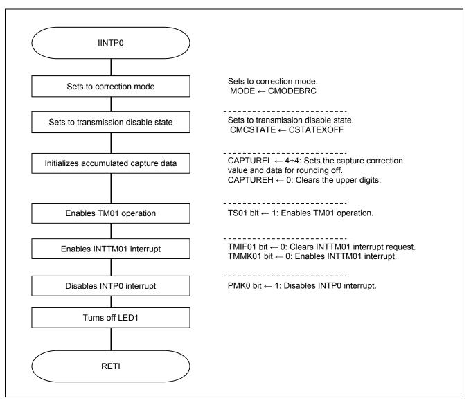
Figure 5.27 INTPO Interrupt Processing
