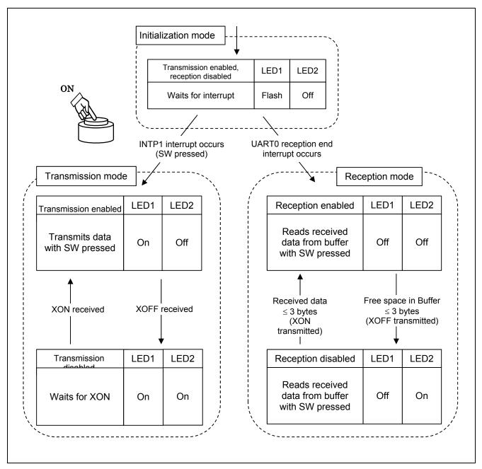
Figure 1.5 State Transition Diagram (Baud Rate Correction Disabled)
