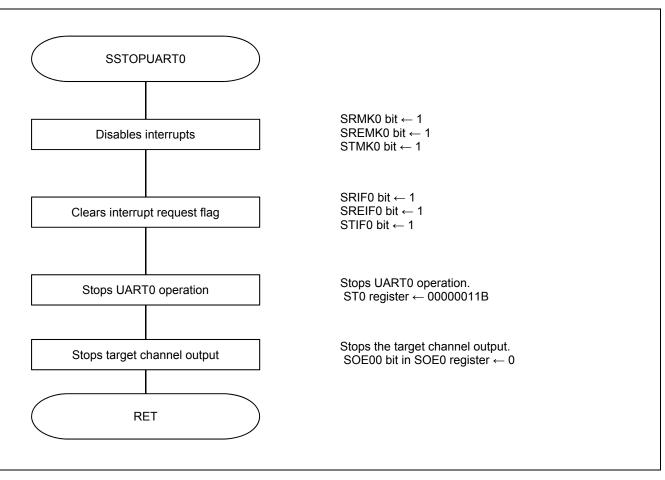
Figure 5.14 UARTO Operation Stop Processing
