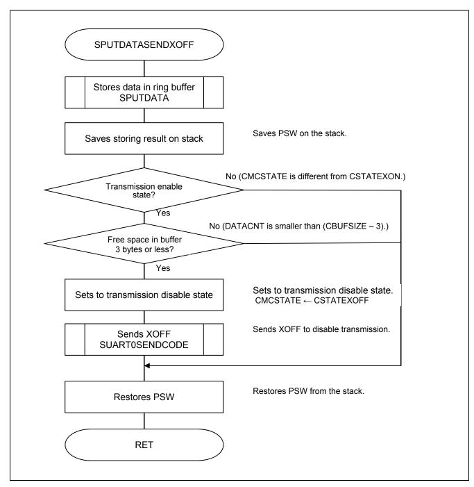
Figure 5.18 Ring Buffer Store and XOFF Transmission Processing
