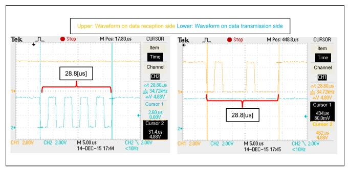
Figure 6.7 Waveforms on Data Transmission Side (Left) and Data Reception Side (Right) (312500bps)
