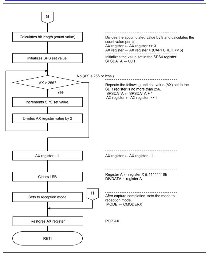
Figure 5.26 INTTM01 Interrupt Processing (2 of 2)
