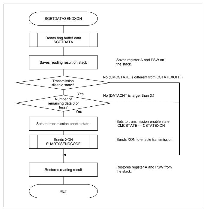
Figure 5.20 Ring Buffer Read and XON Transmission Processing
