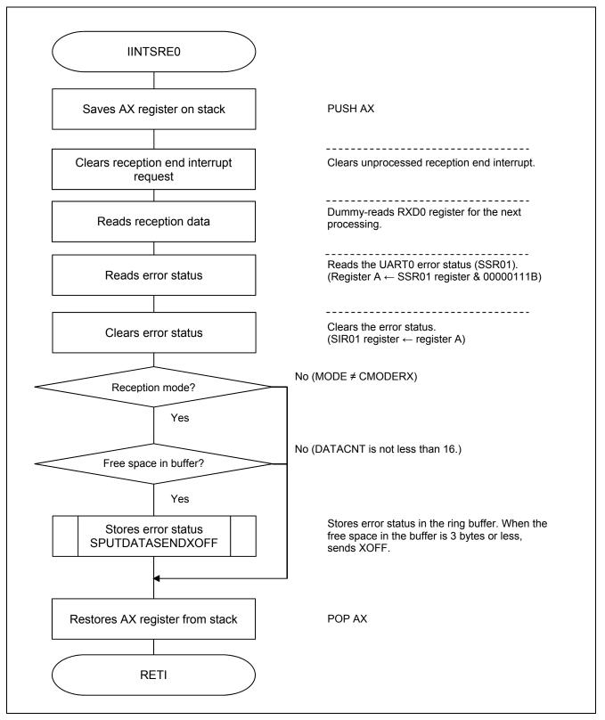
Figure 5.23 UARTO Reception Error Interrupt Processing
