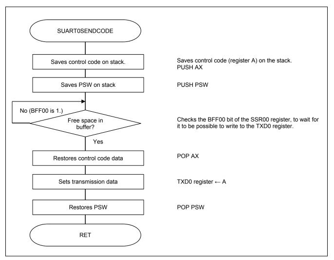
Figure 5.16 UART0 Control Code Transmission Processing
