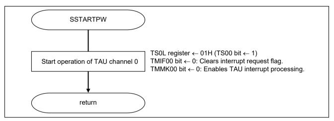
Figure 5.7 Timer Array Unit Startup
