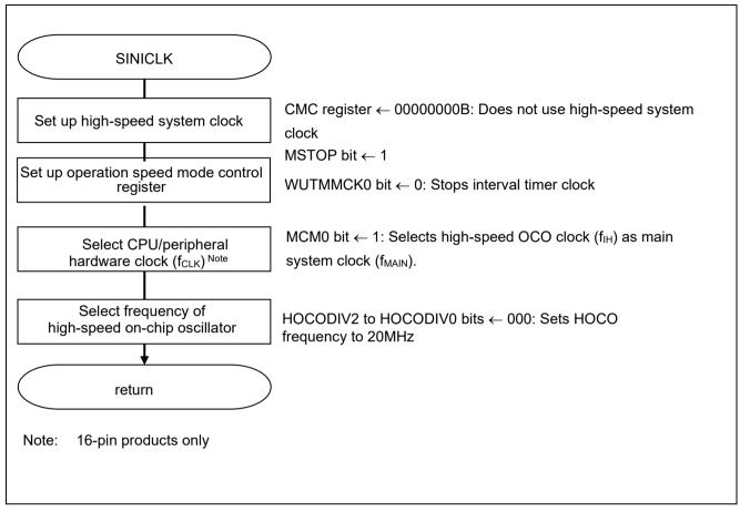
Figure 5.4 Clock Generation Circuit Setup
