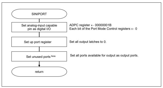
Figure 5.3 I/O Port Setup
