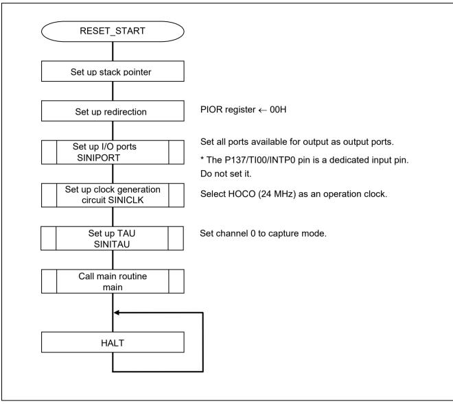
Figure 5.2 CPU Initialization Function
