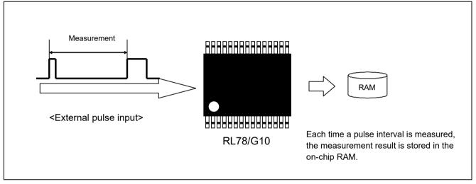
Figure 1.1 Outline of Pulse Interval Measurement
