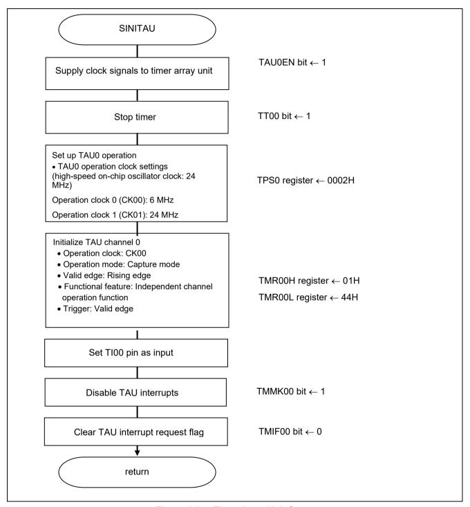
Figure 5.5 Timer Array Unit Setup
