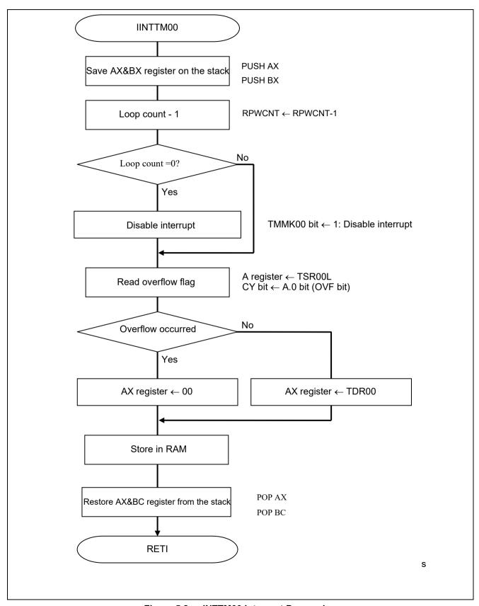
Figure 5.8 INTTM00 Interrupt Processing
