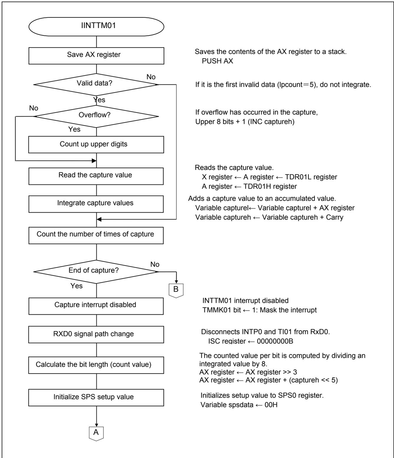
**Figure 5.8 Completion of INTTM01 Capture Interrupt Processing (1/2)**
