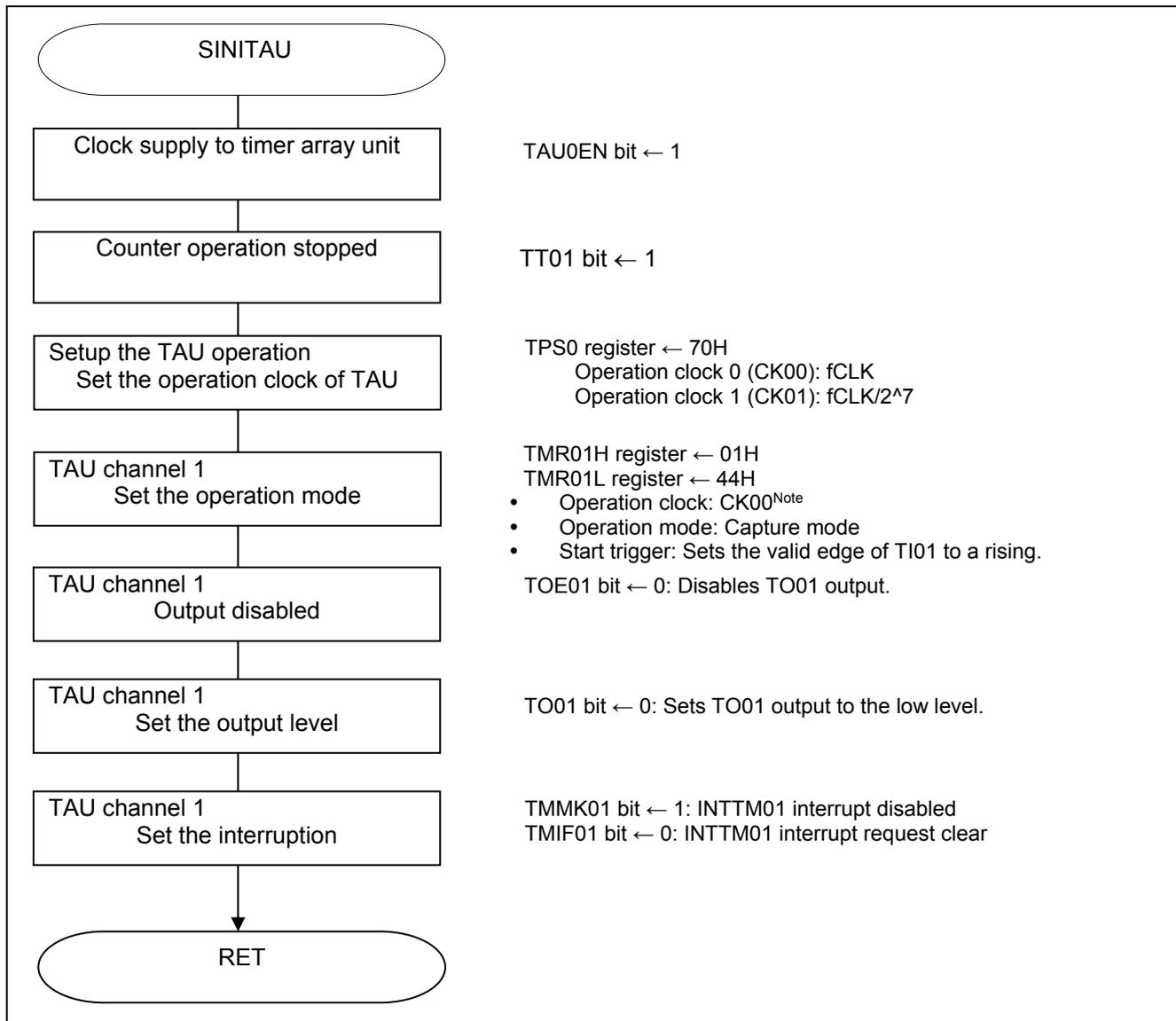
**Figure 5.5 Setup of Timer Array Unit**
