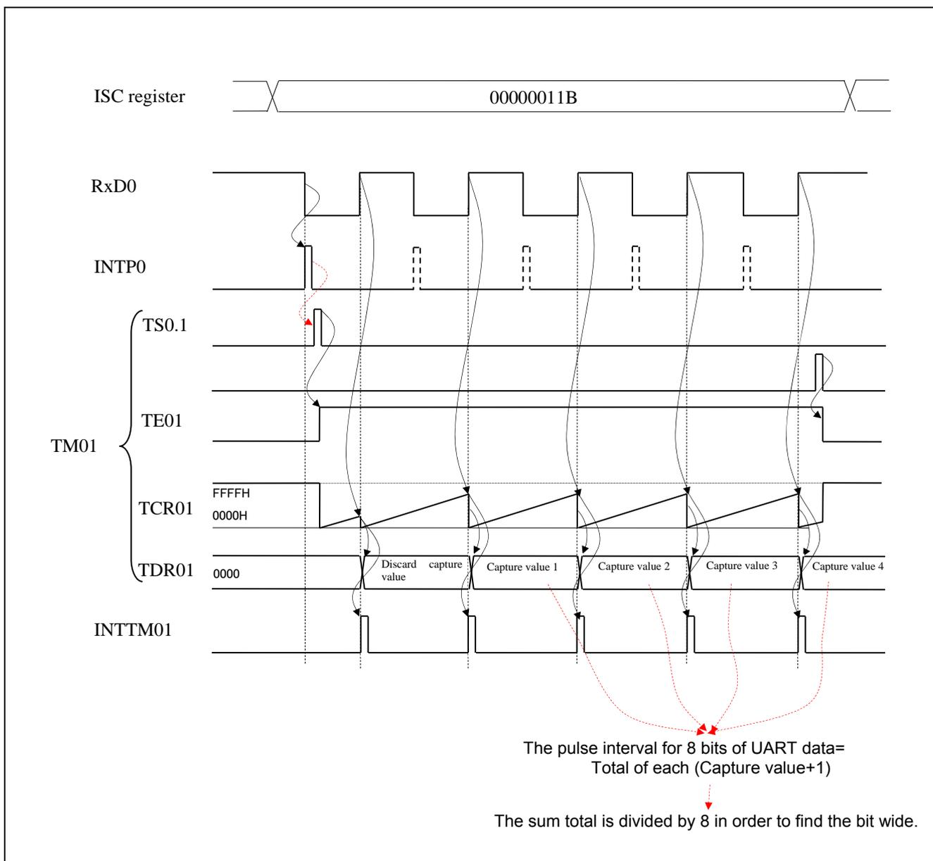
**Figure 1.2 Timing Chart of Baud Rate Measurement**
