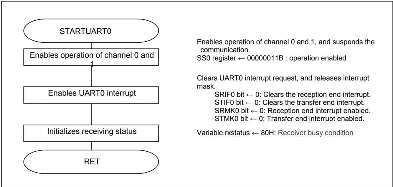
Figure 5.9 Enabling UART0 Operation
