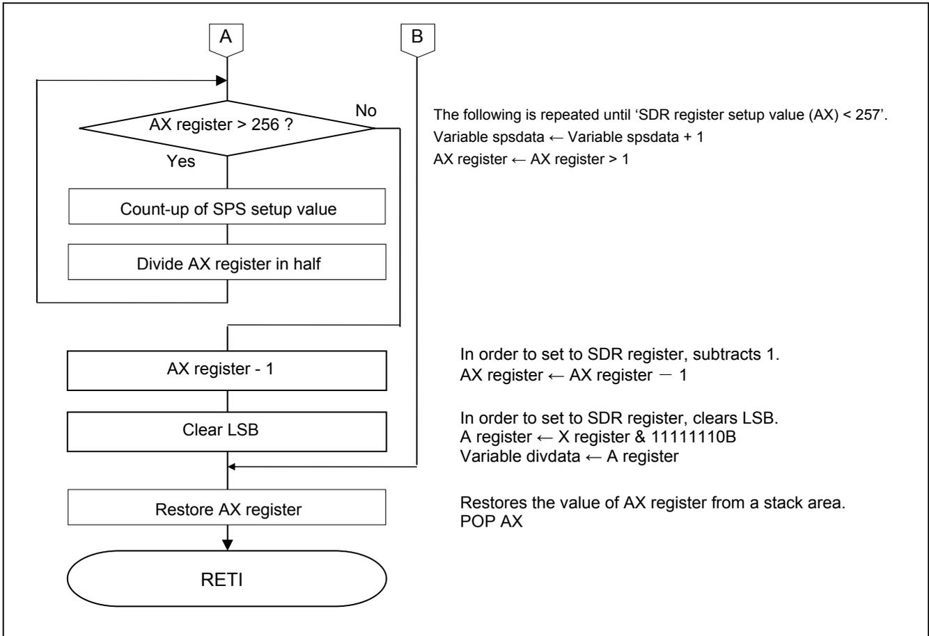
Figure 5.8 Completion of INTTM01 Capture Interrupt Processing (2/2)
