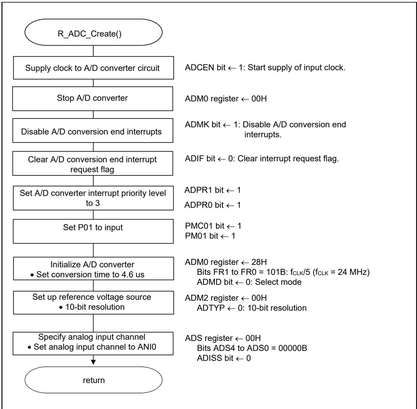
Figure 5.6 A/D Converter Setup Flowchart
