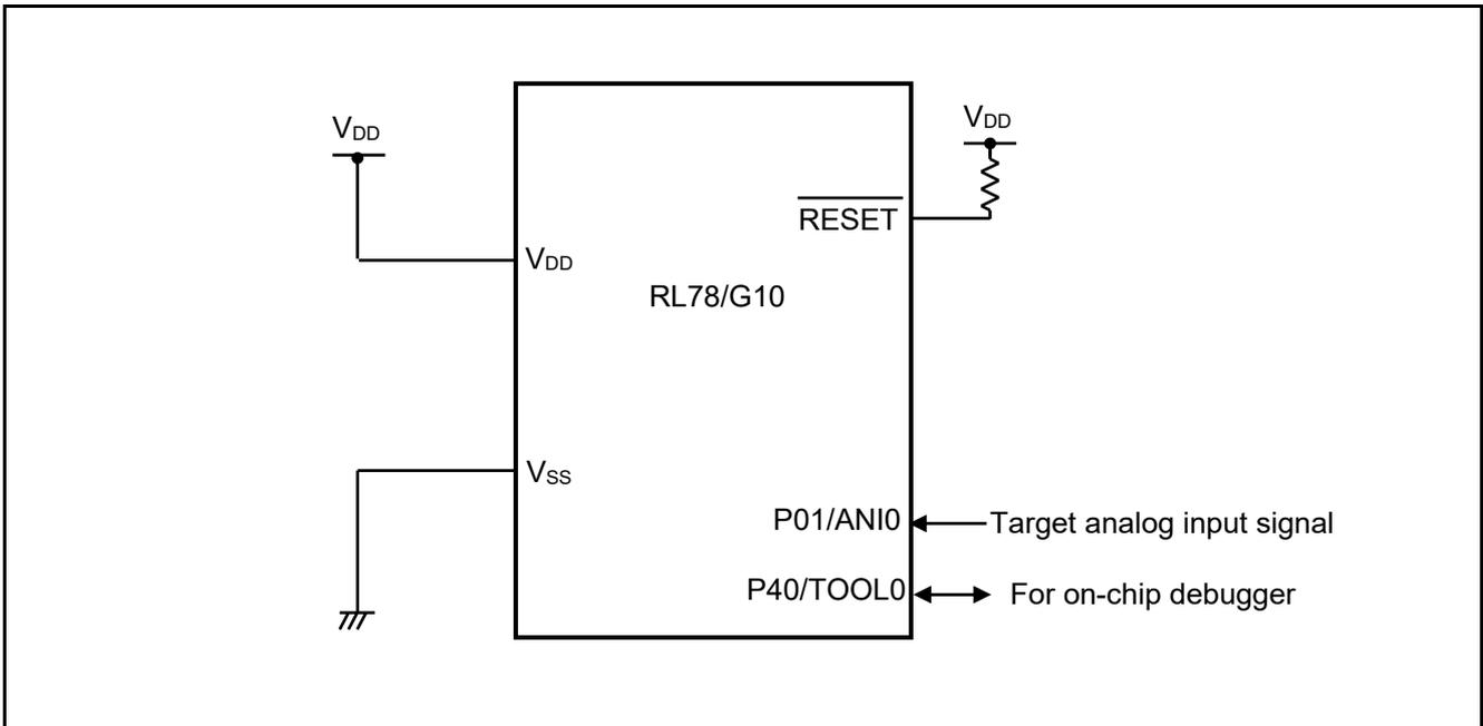
**Figure 4.1 Hardware Configuration**
