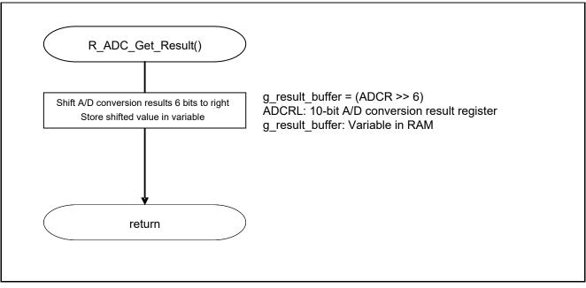
Figure 5.11 Storing the A/D Conversion Results in RAM
