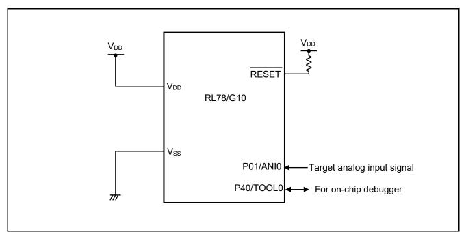
Figure 4.1 Hardware Configuration
