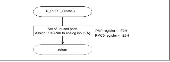
Figure 5.4 I/O Port Setup
