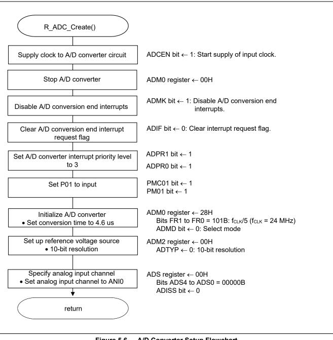
Figure 5.6 A/D Converter Setup Flowchart
