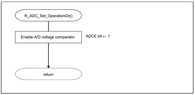
Figure 5.9 Enabling the A/D Voltage Comparator
