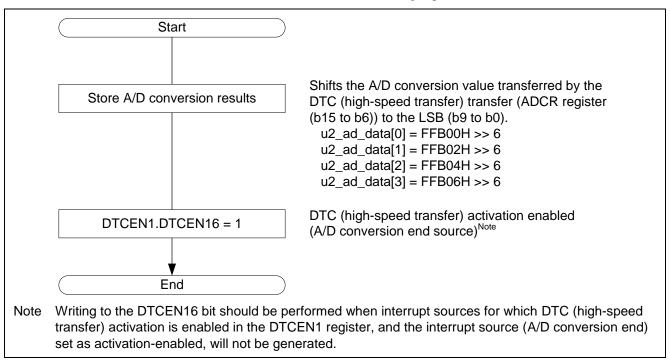
Figure 3.6 DTC (High-Speed Transfer) Transfer-End Interrupt (A/D Conversion End Interrupt)
