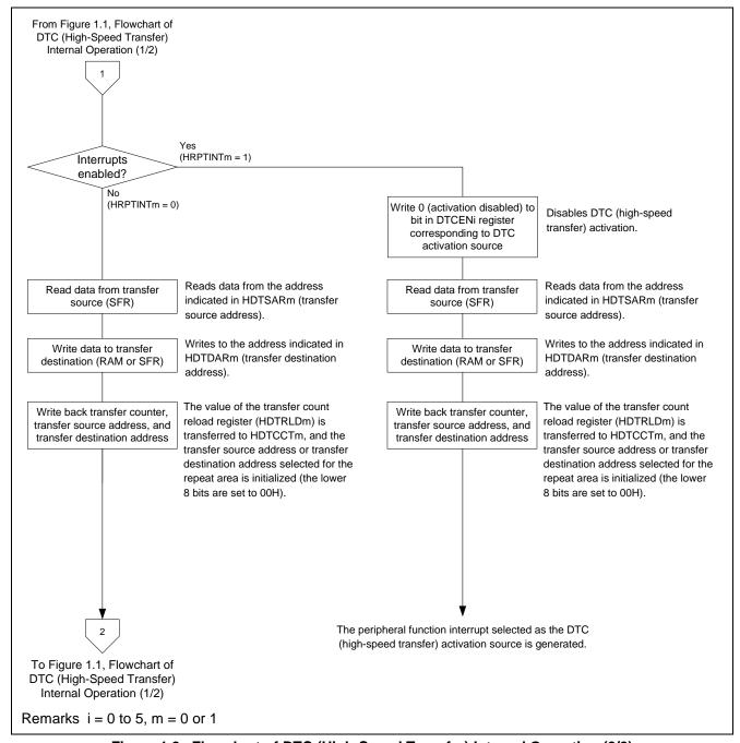
Figure 1.2 Flowchart of DTC (High-Speed Transfer) Internal Operation (2/2)
