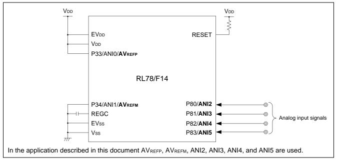
Figure 2.1 Connection Diagram of Pins Used
