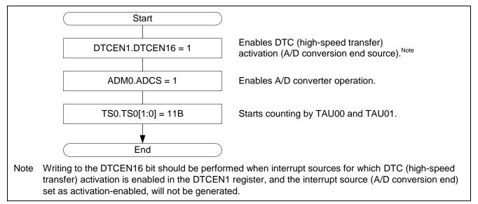
Figure 3.5 Procedure for Enabling Peripheral Functions (DTC (High-Speed Transfer) Transfer Start)
