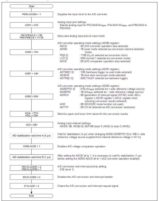
Figure 3.3 A/D Converter Initialization Procedure
