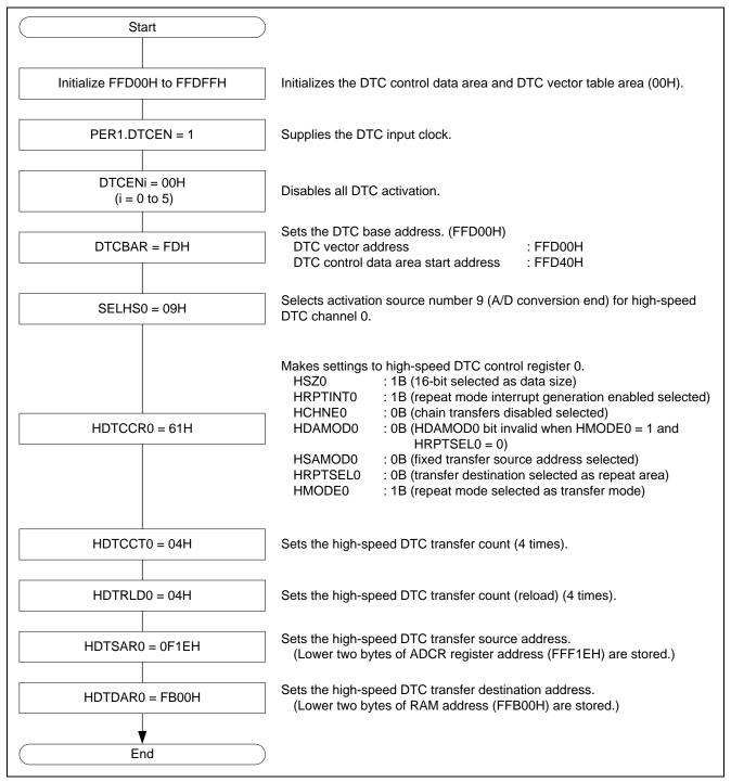
Figure 3.2 DTC (High-Speed Transfer) Initialization Procedure
