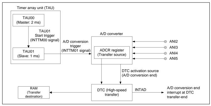
Figure 2.2 Configuration Diagram of Peripheral Functions Used
