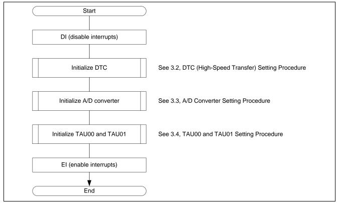
Figure 3.1 Peripheral Function Initialization Procedure
