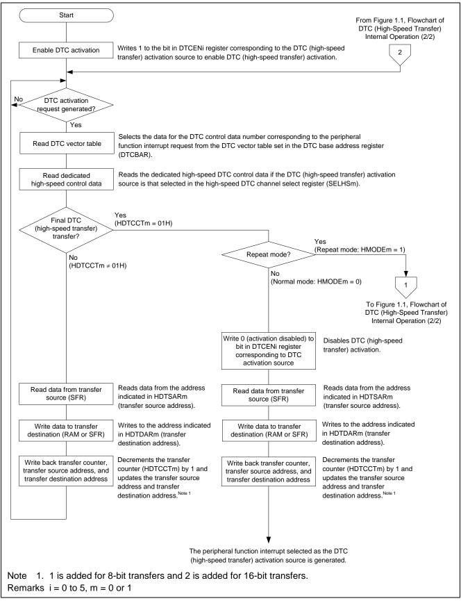
Figure 1.1 Flowchart of DTC (High-Speed Transfer) Internal Operation (1/2)
