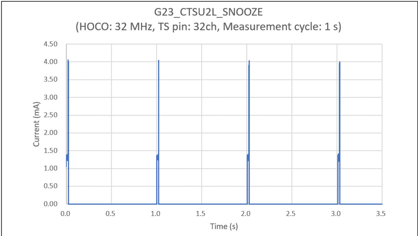
Figure 5 - 7 Current consumption waveform: TS pin 32ch measurement (2/2)
