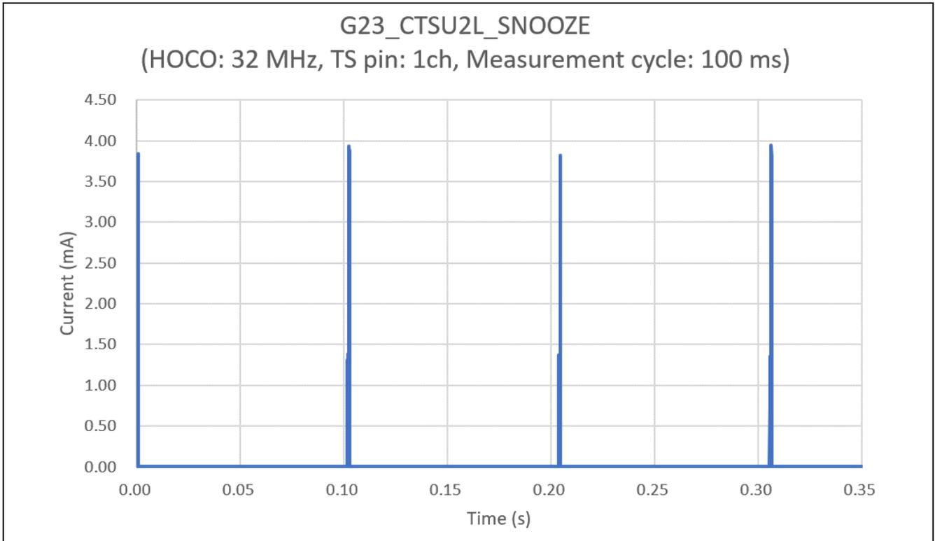
Figure 5 - 5 Current consumption waveform: TS pin 1ch measurement (2/2)
