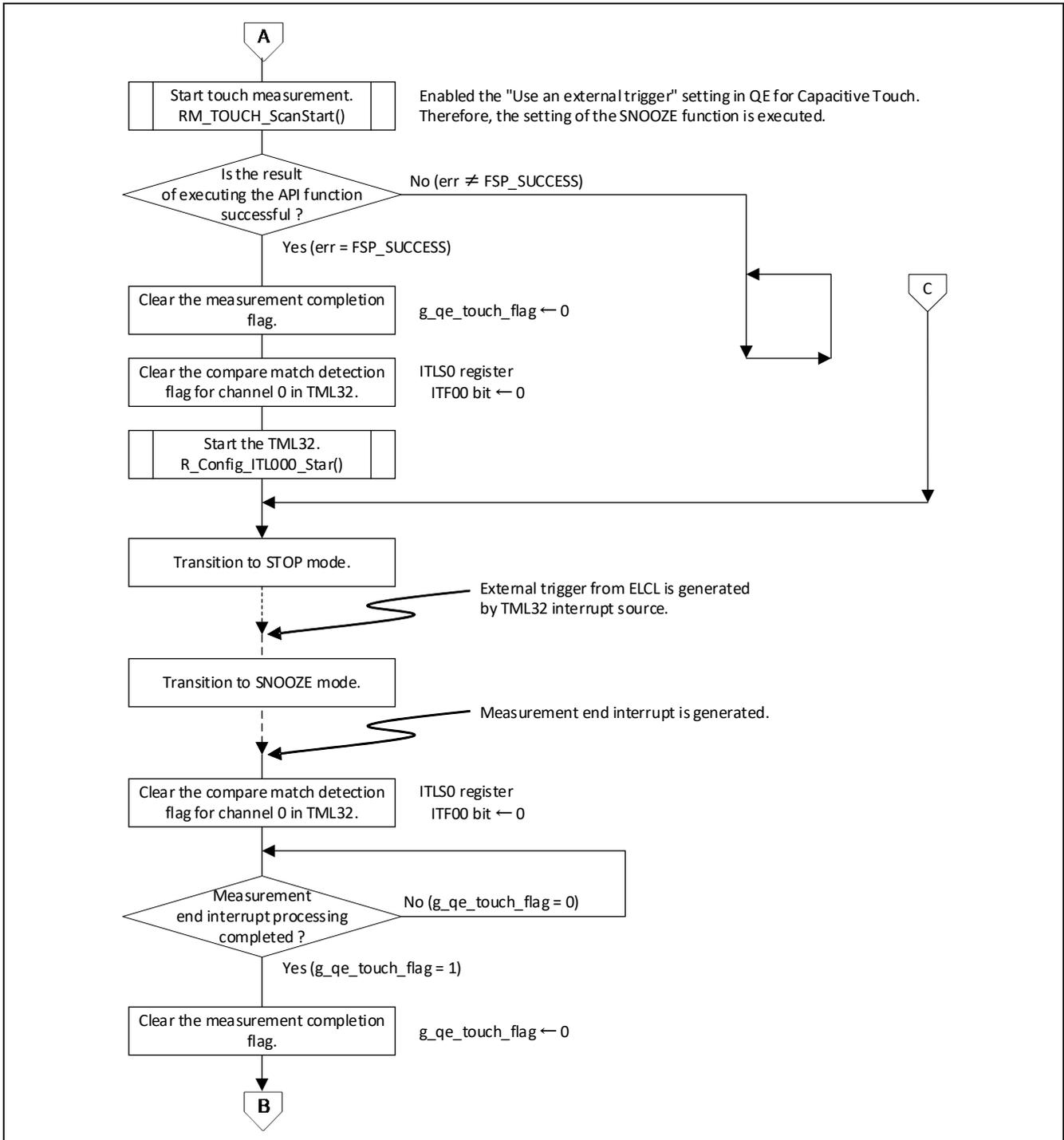
Figure 4 - 4 Touch measurement control processing (3/3)
