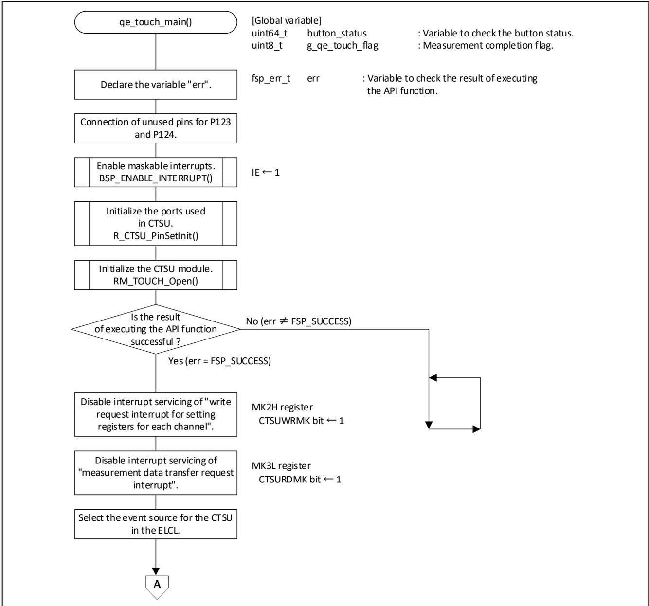
Figure 4 - 3 Touch measurement control processing (2/3)
