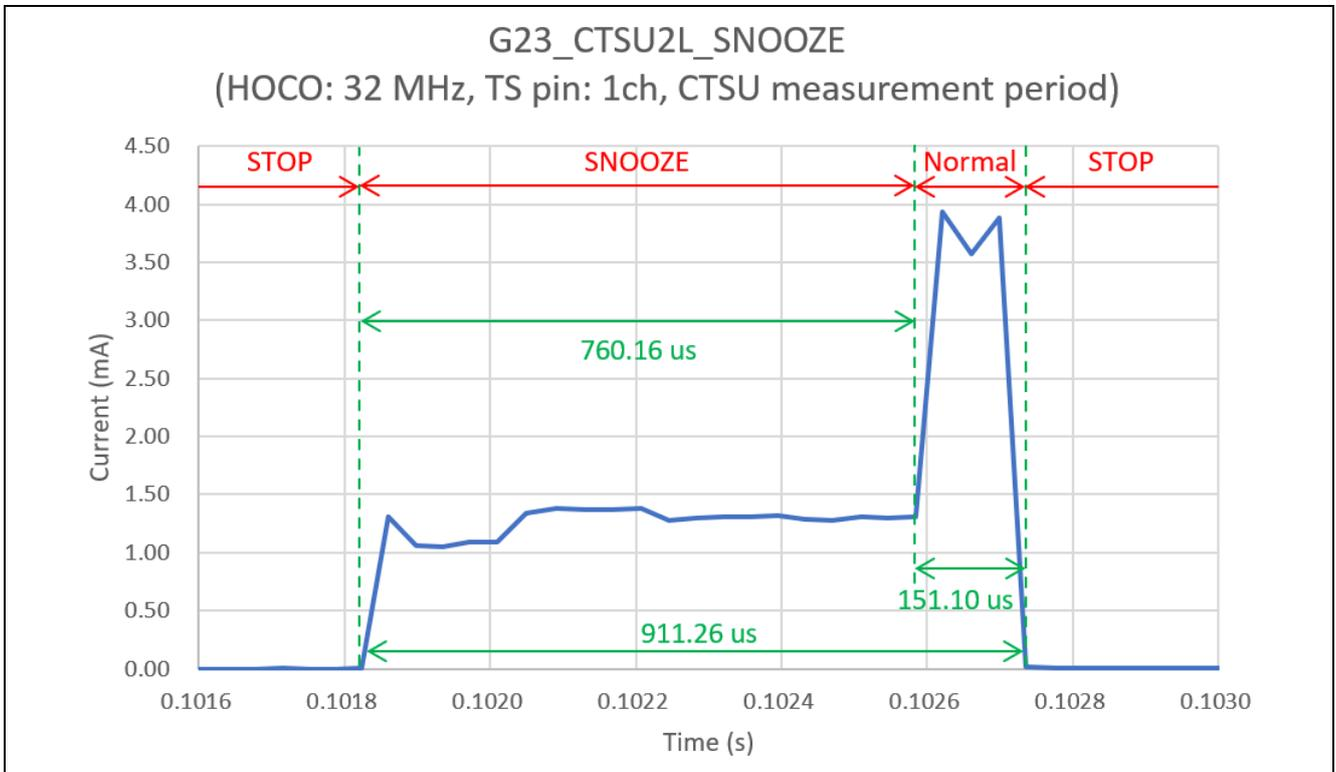
Figure 5 - 6 Current consumption waveform: TS pin 32ch measurement (1/2)
