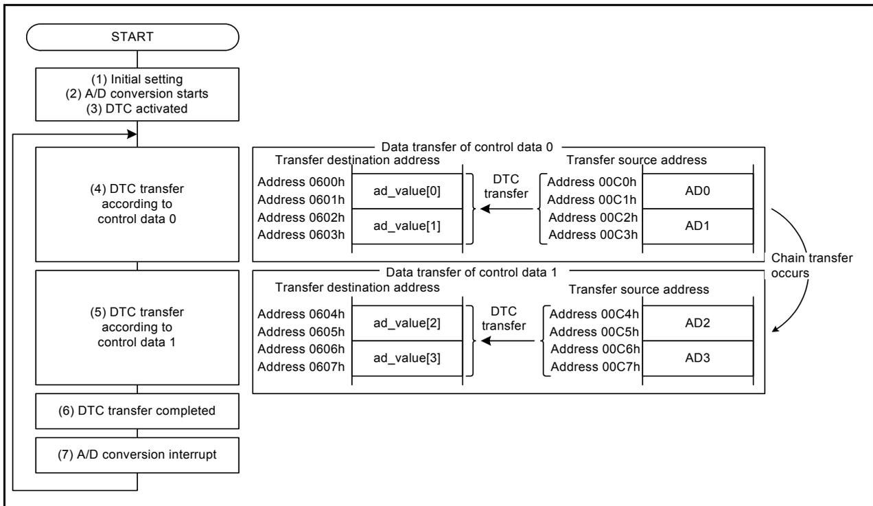
Figure 4.1 Example of Chain Transfer
