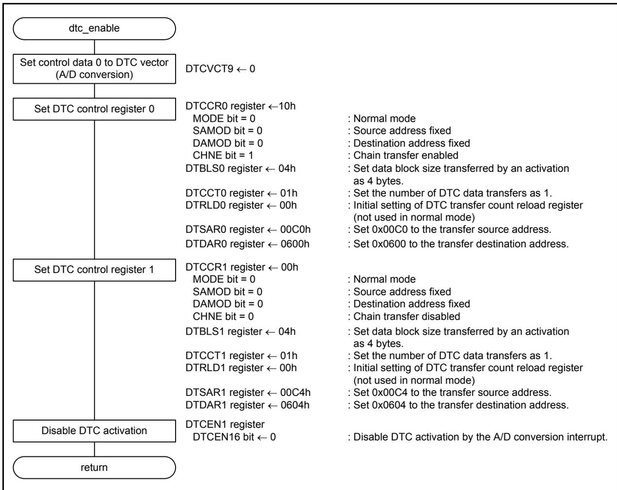
Figure 4.5 Initial Setting of the DTC
