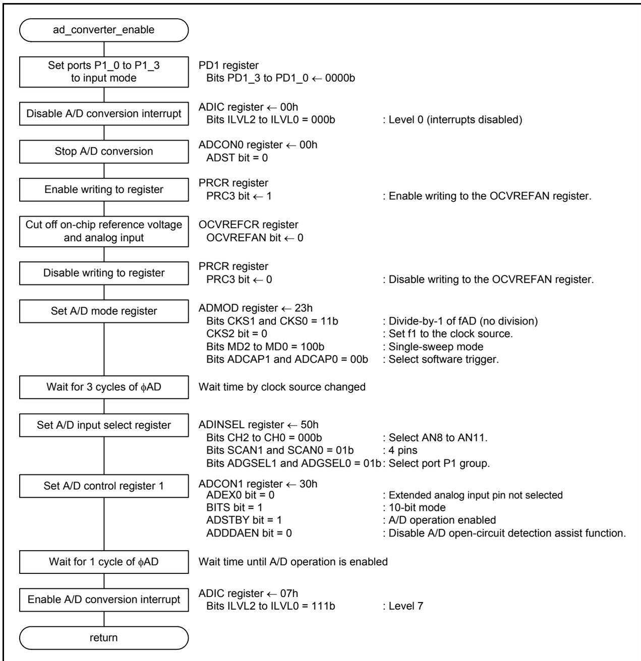
Figure 4.4 Initial Setting of the A/D Converter
