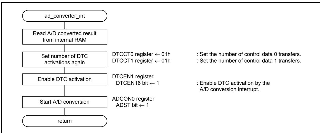
**Figure 4.6 A/D Conversion Interrupt Handling**
