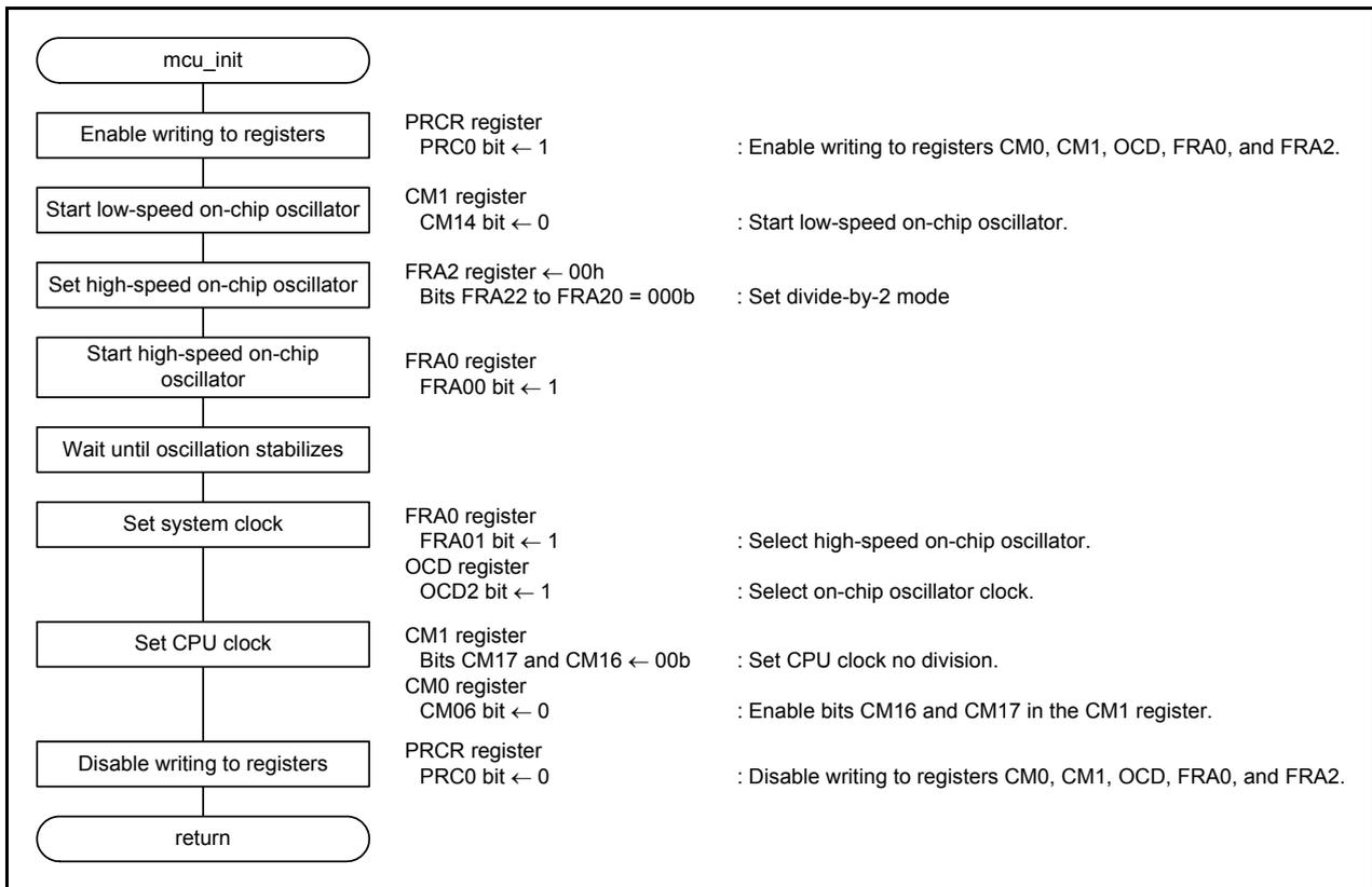
**Figure 4.3 System Clock Setting**
