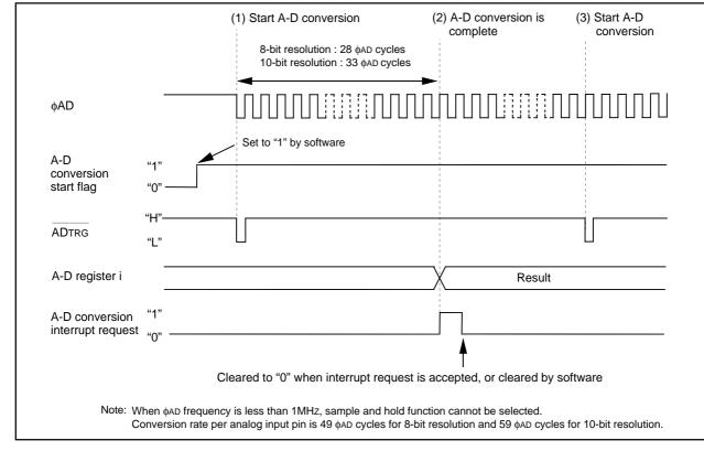
Figure 1. Operation timing of one-shot mode, with an external trigger selected
